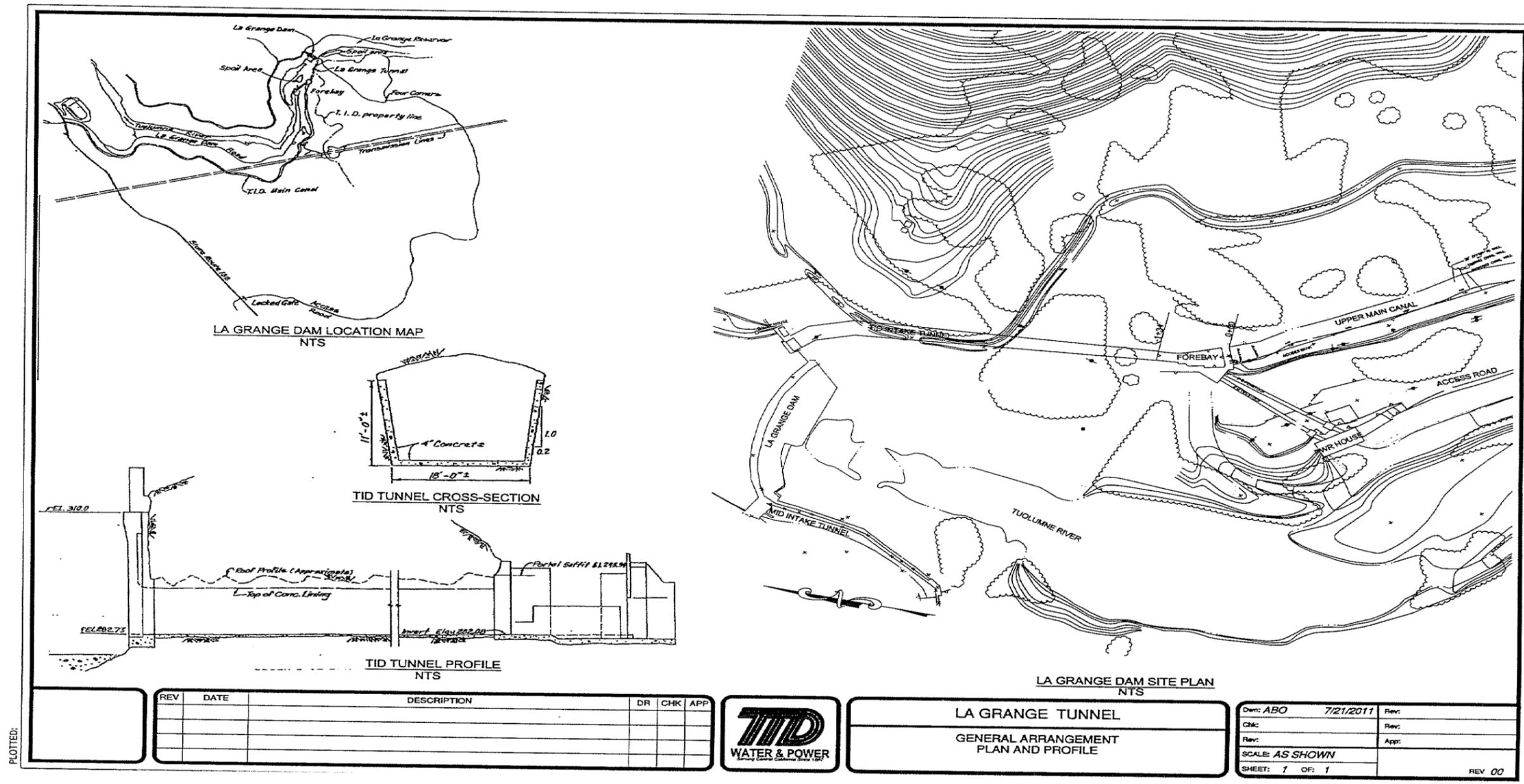
Figure 1. Site plan of La Grange diversion dam and facilities showing diversion dam, TID tunnel intake, tunnel location, penstocks, powerhouse, and Upper Main Canal.
