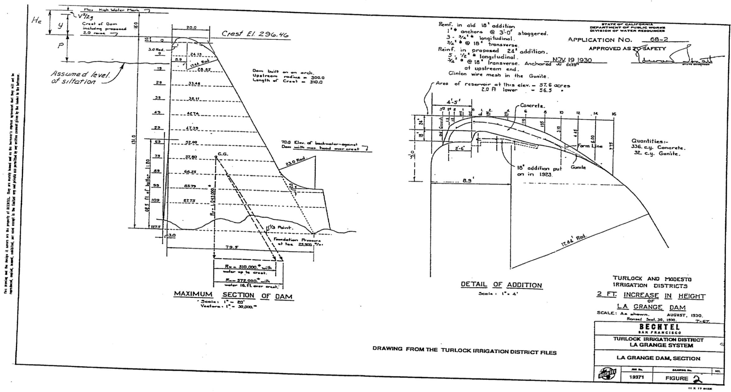
Figure 2. La Grange spillway section showing original crest and crest modification to present elevation of 296.5 feet.
