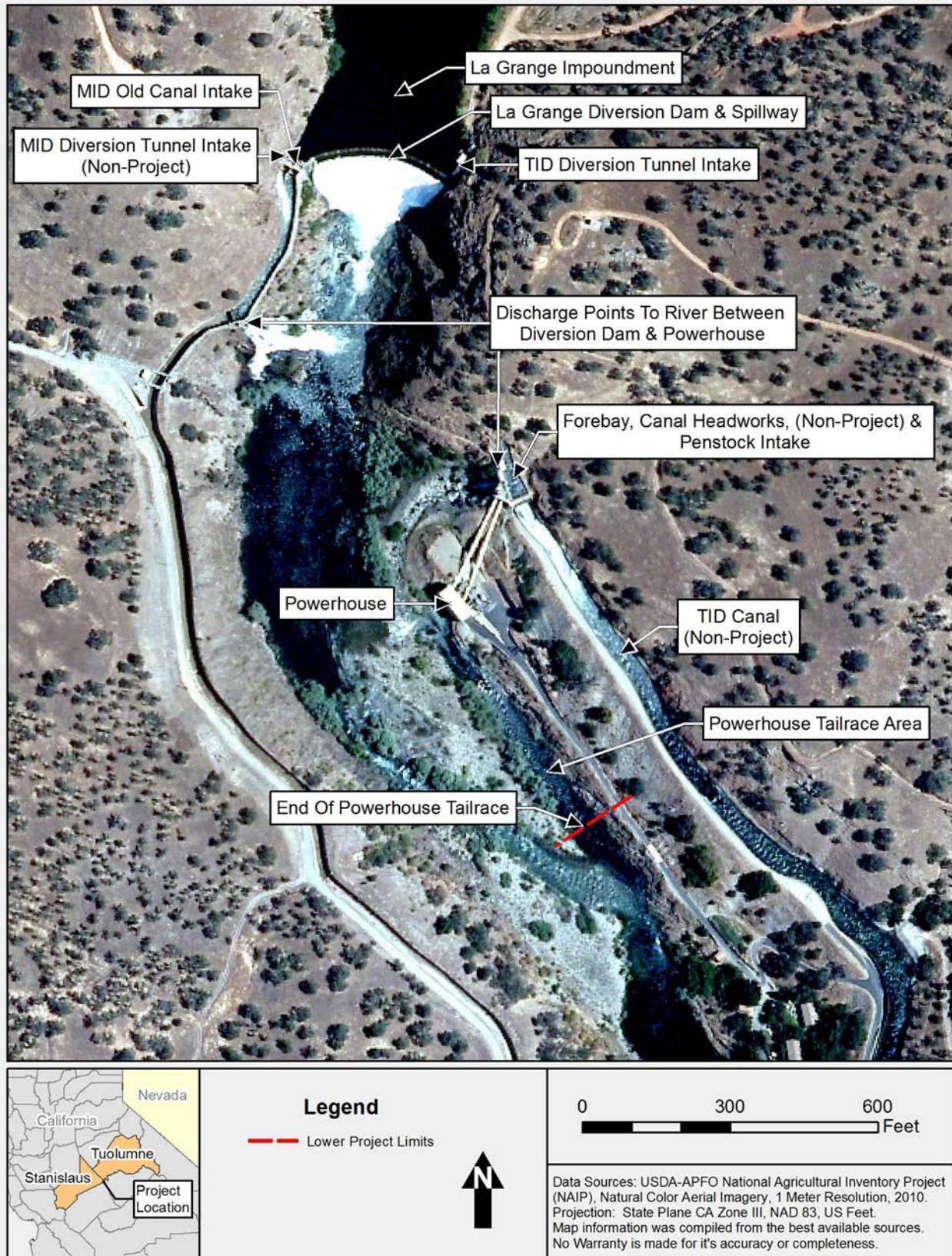
Figure 1.1-2. La Grange Hydroelectric Project site plan.
