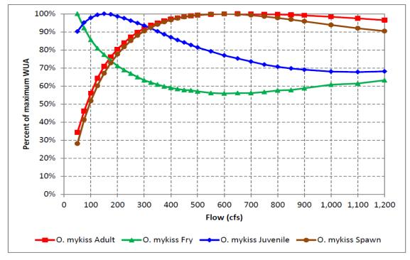
Figure 3.3.2-23. *O. mykiss* WUA versus flow for the lower Tuolumne River (Source: Stillwater Sciences, 2013c).
