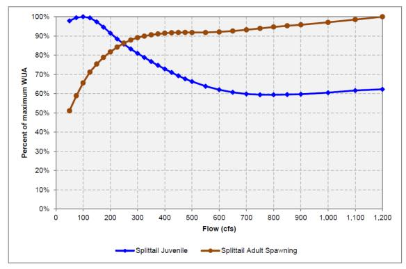
Figure 3.3.2-25. Sacramento splittail WUA versus flow for the lower Tuolumne River (Source: Stillwater Sciences, 2014).
