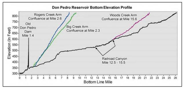
Figure 3.3.2-22. Don Pedro Reservoir bottom elevation profile including the crest of the old dam (Source: HDR, 2017b).
