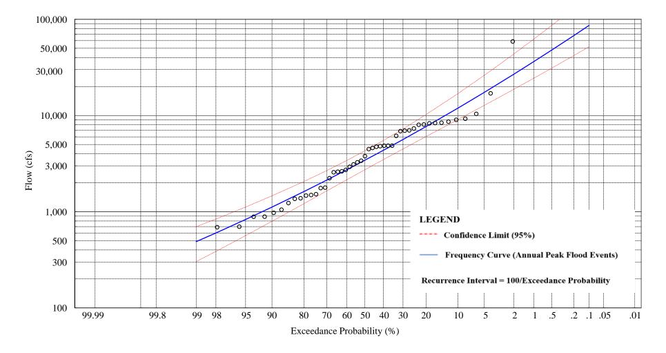
Figure 3.3.1-1. Flood frequency curve (peak annual flood) for the La Grange gage, 1971–2017 (Source: USGS, 2018a).
