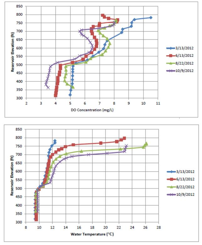
Figure 3.3.2-9. DO concentration and water temperature vertical profiles recorded in Don Pedro Reservoir near the dam in 2012 (Source: Districts, 2017a).
