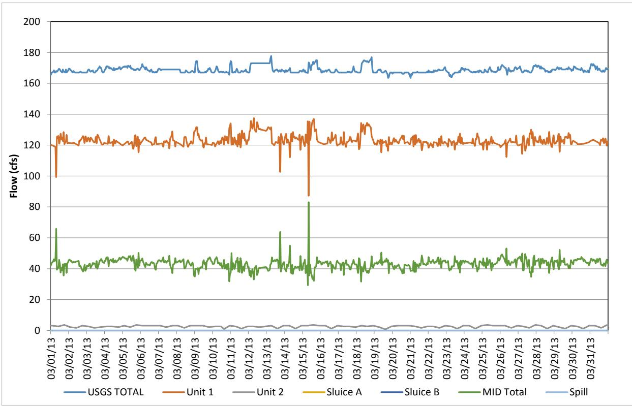
**Figure D-99.** Flow record in March 2013, based on hourly discharges.
