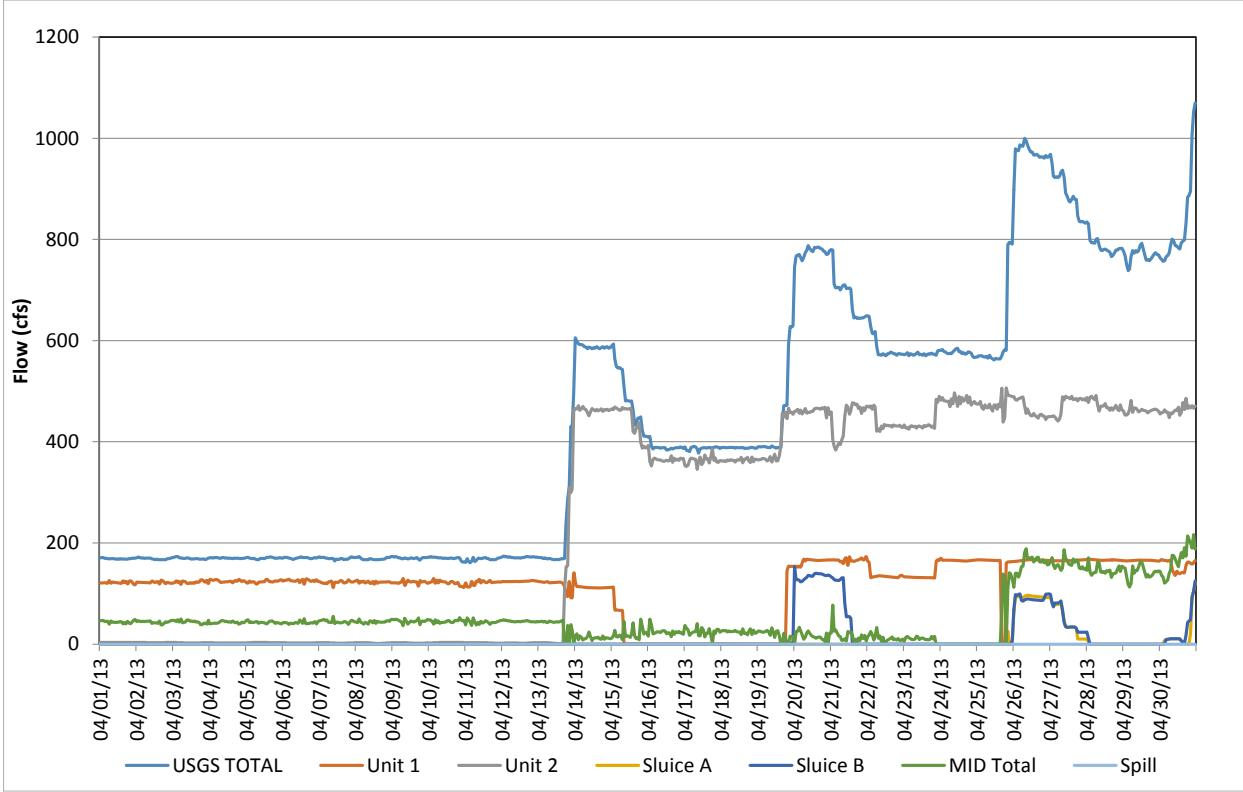
**Figure D-100.** Flow record in April 2013, based on hourly discharges.
