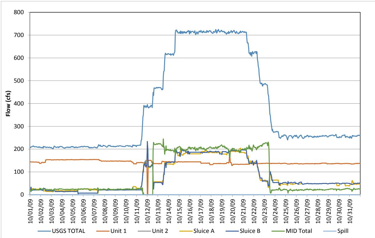
**Figure D-58.** Flow record in October 2009, based on hourly discharges.
