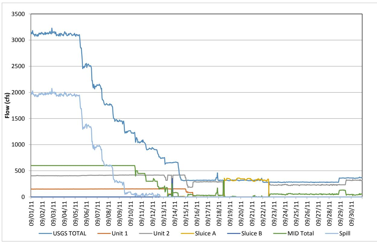
**Figure D-81.** Flow record in September 2011, based on hourly discharges.
