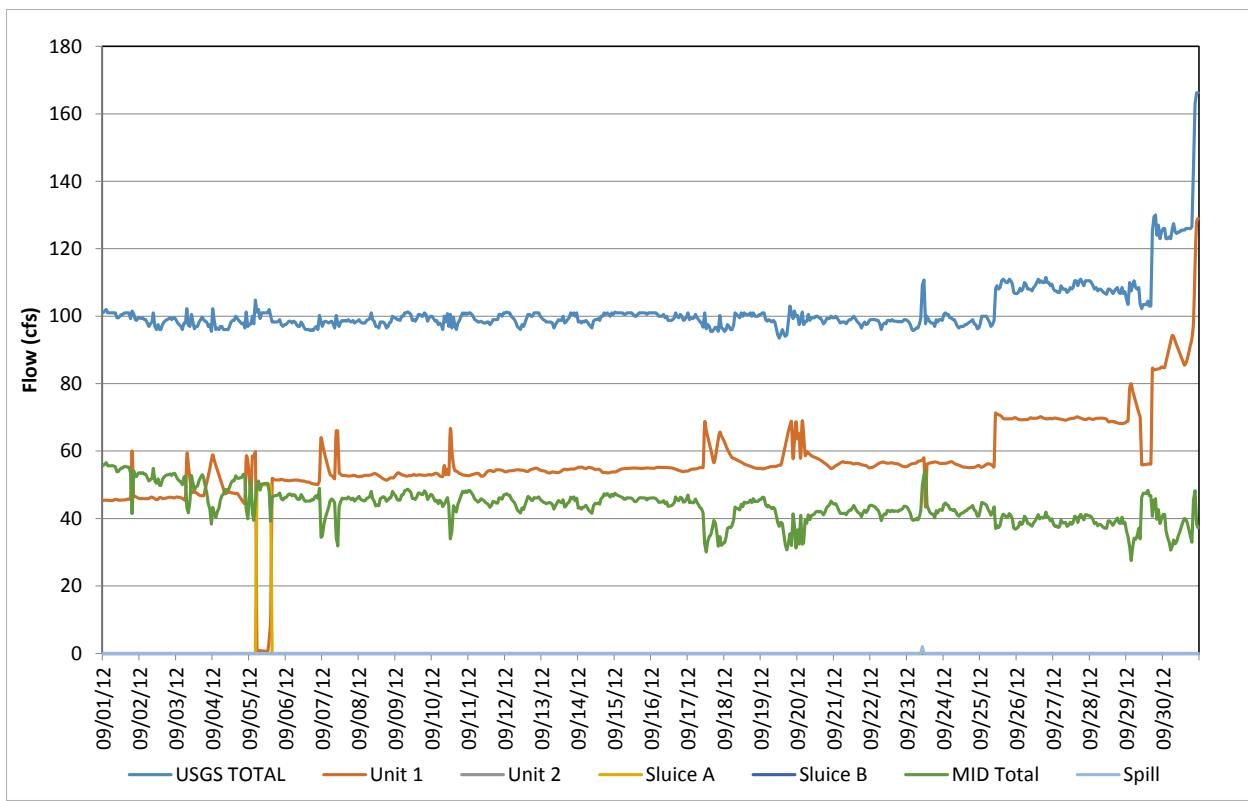
**Figure D-93.** Flow record in September 2012, based on hourly discharges.
