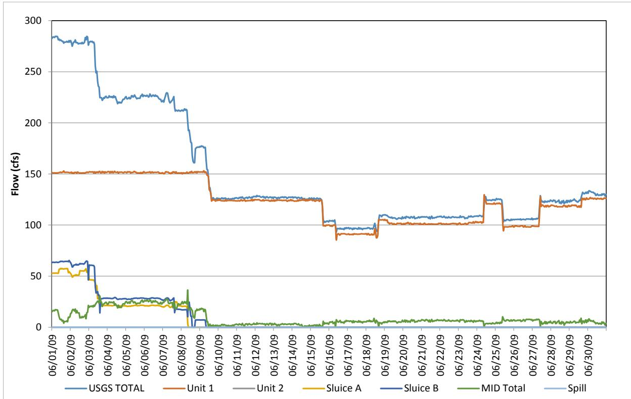
**Figure D-54.** Flow record in June 2009, based on hourly discharges.
