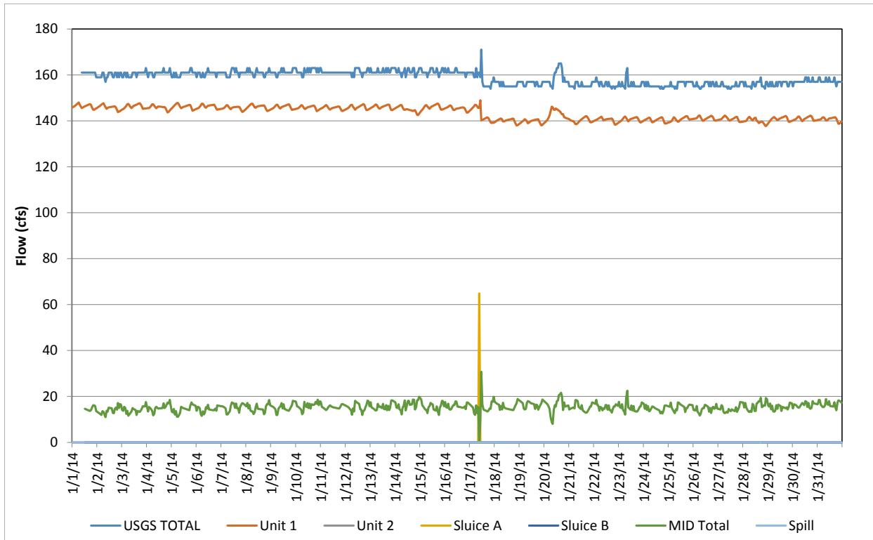
**Figure A-1.** Flow record in January 2014, based on hourly discharges.
