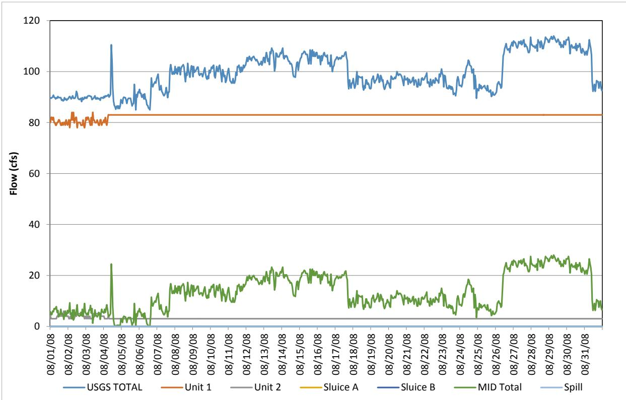
**Figure D-44.** Flow record in August 2008, based on hourly discharges.
