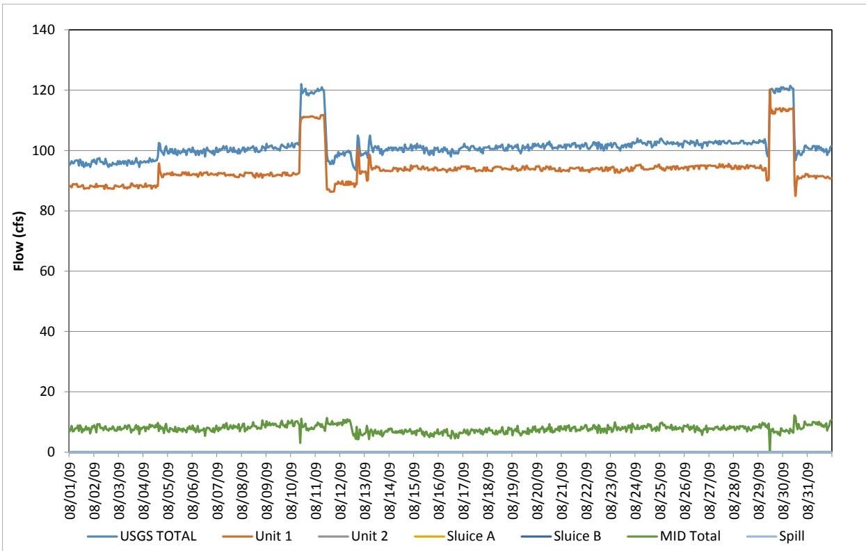
**Figure D-56.** Flow record in August 2009, based on hourly discharges.
