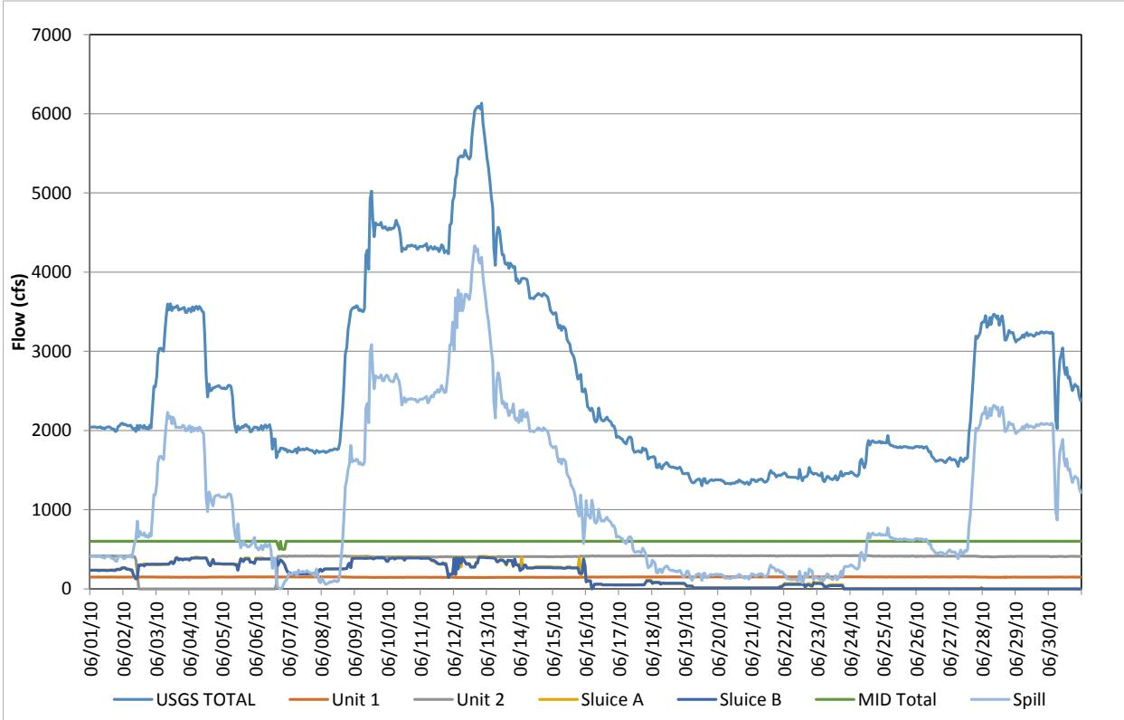
**Figure D-66.** Flow record in June 2010, based on hourly discharges.
