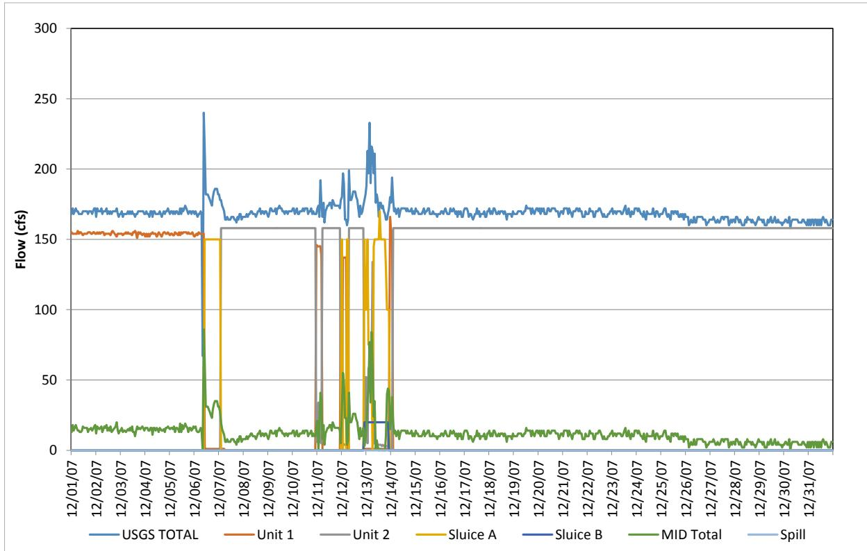
**Figure D-36.** Flow record in December 2007, based on hourly discharges.
