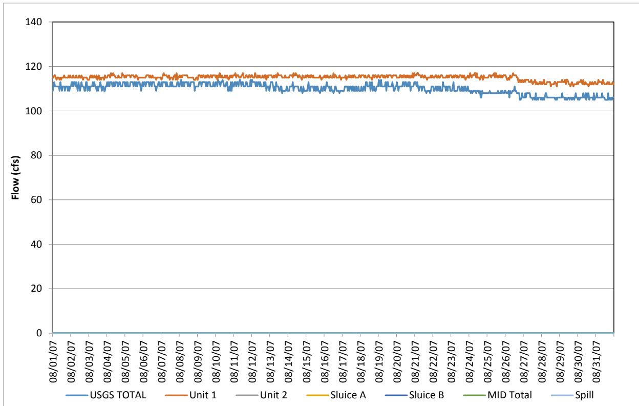
**Figure D-32.** Flow record in August 2007, based on hourly discharges.
