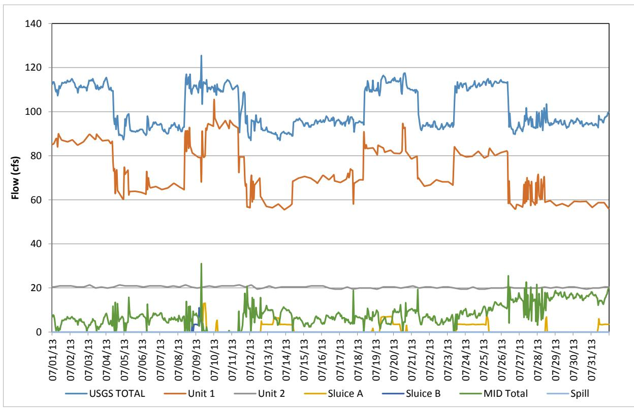
**Figure D-103.** Flow record in July 2013, based on hourly discharges.
