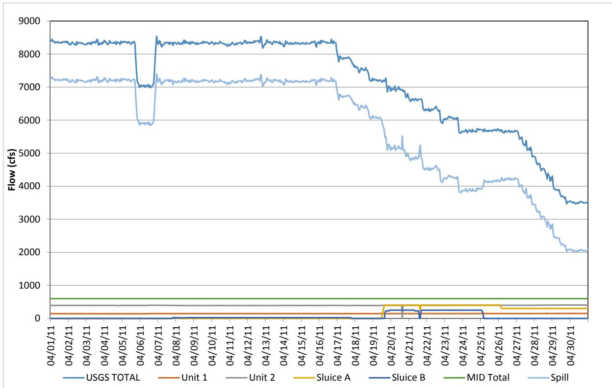
**Figure D-76.** Flow record in April 2011, based on hourly discharges.
