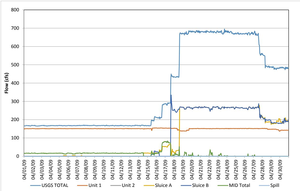
**Figure D-52.** Flow record in April 2009, based on hourly discharges.
