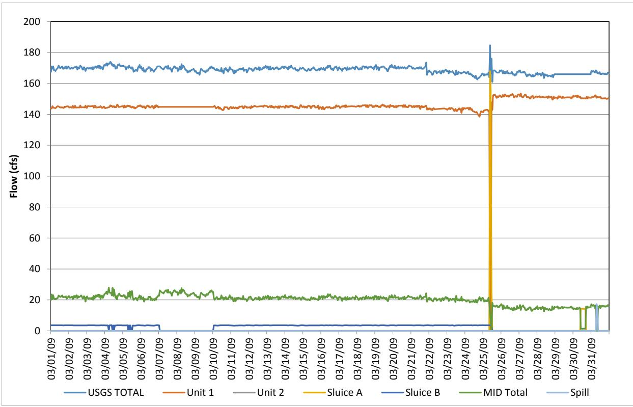
**Figure D-51.** Flow record in March 2009, based on hourly discharges.
