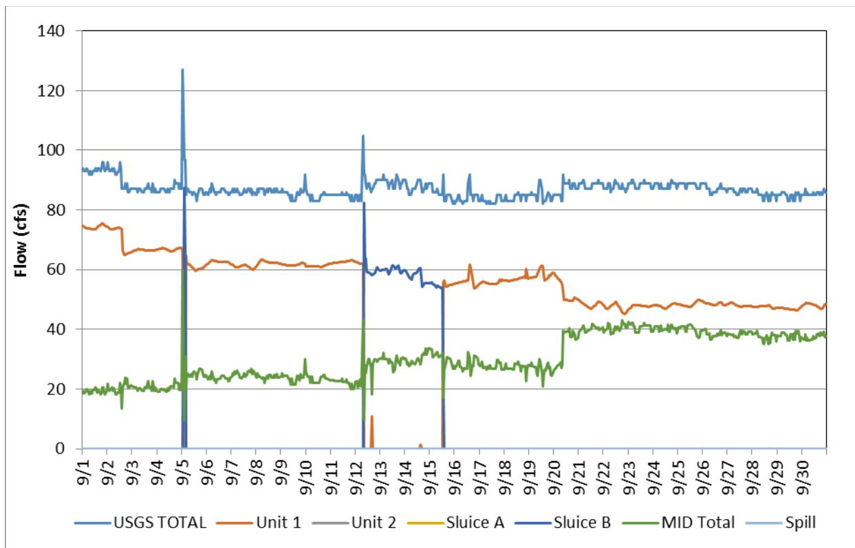
**Figure C-9.** Flow record in September 2016, based on hourly discharges.
