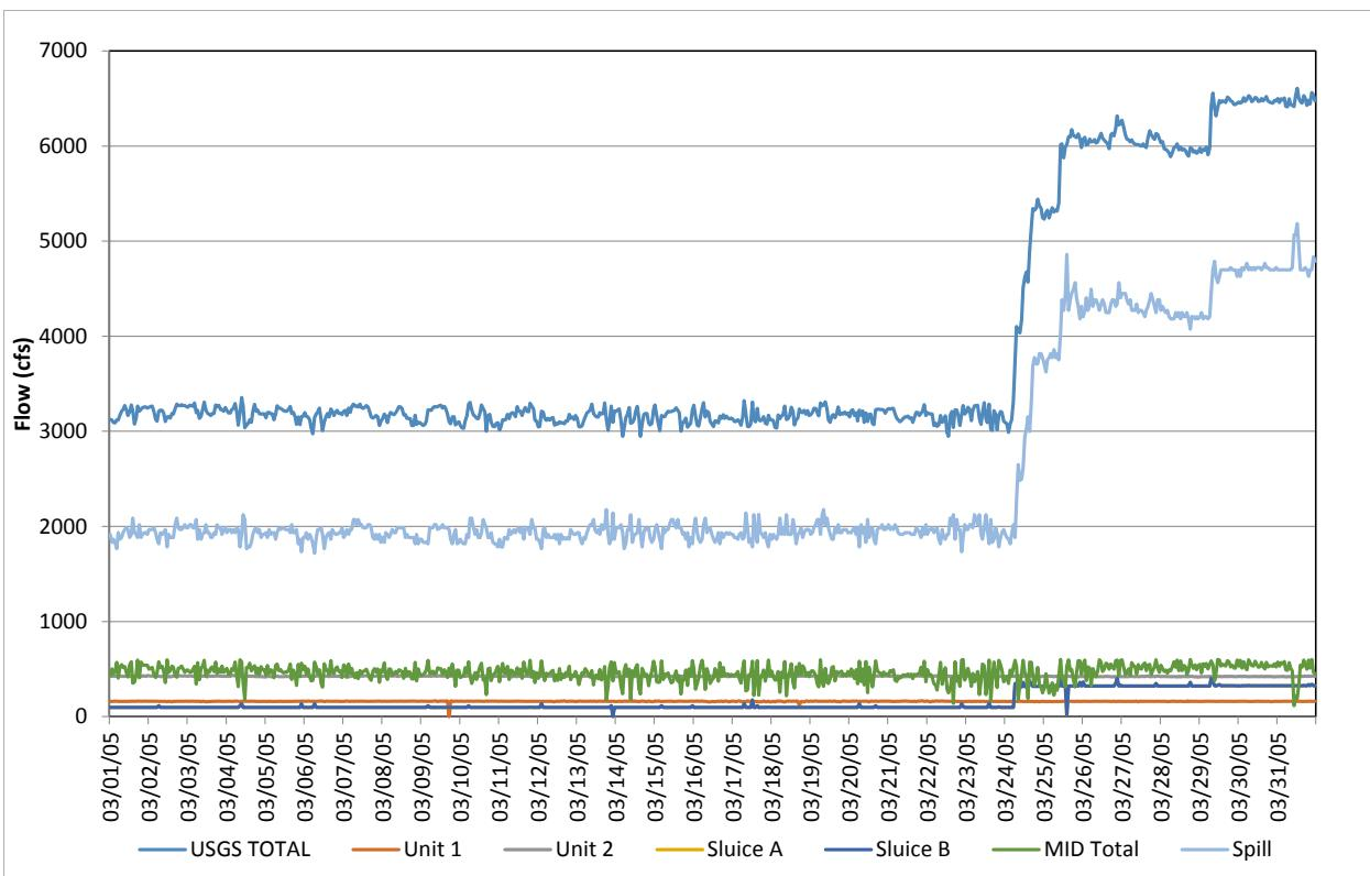
**Figure D-3.** Flow record in March 2005, based on hourly discharges.
