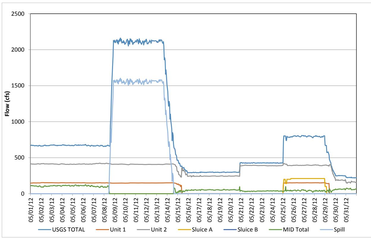
**Figure D-89.** Flow record in May 2012, based on hourly discharges.
