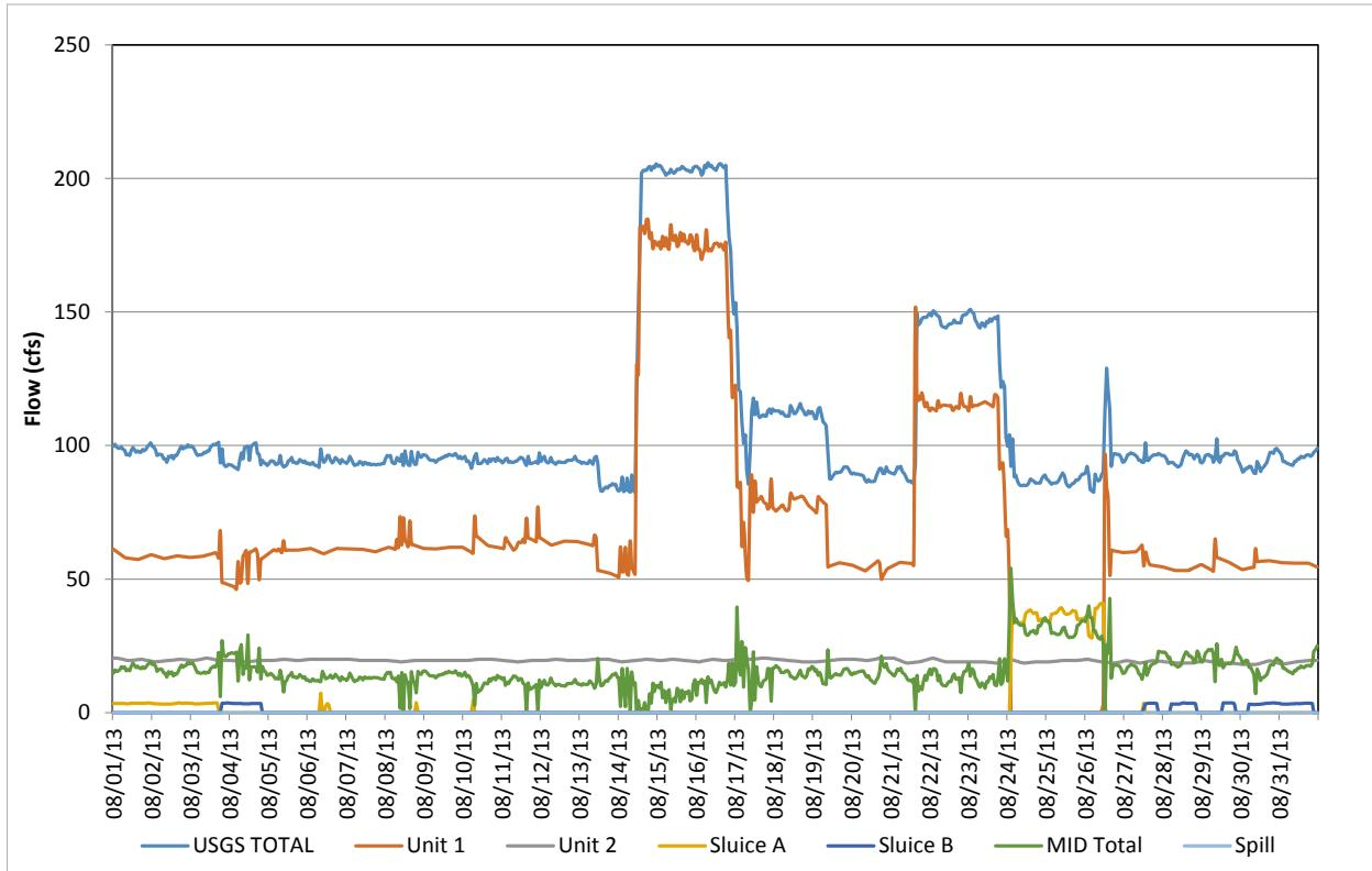
**Figure D-104.** Flow record in August 2013, based on hourly discharges.
