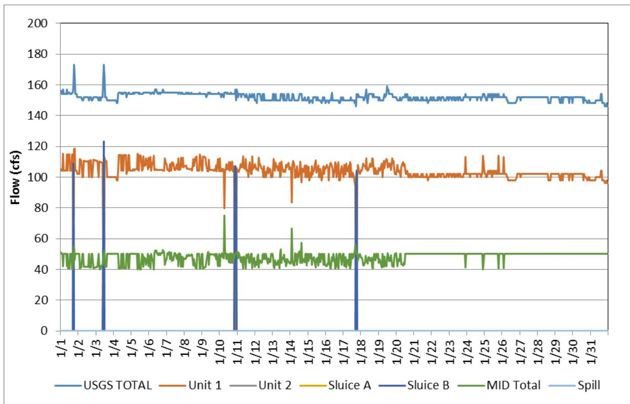
**Figure C-1.** Flow record in January 2016, based on hourly discharges.
