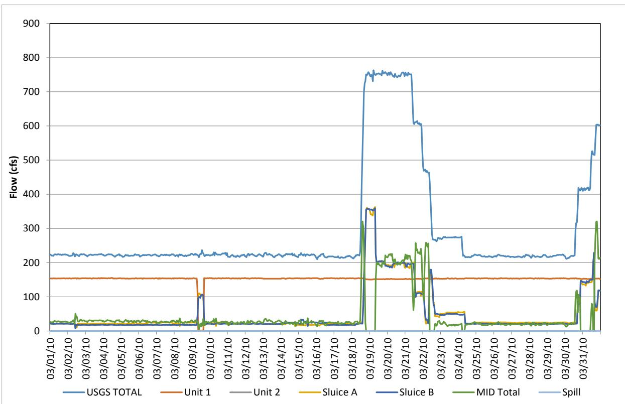
**Figure D-63.** Flow record in March 2010, based on hourly discharges.
