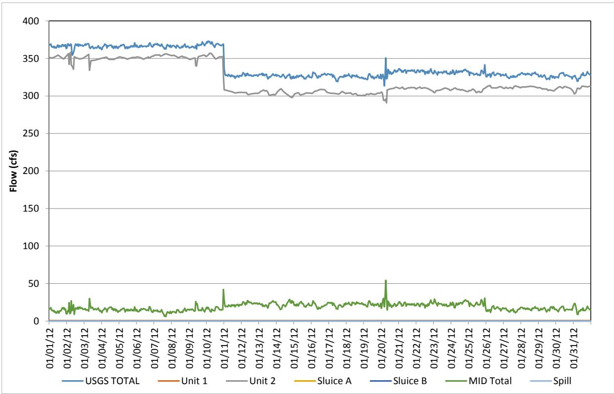
**Figure D-85.** Flow record in January 2012, based on hourly discharges.
