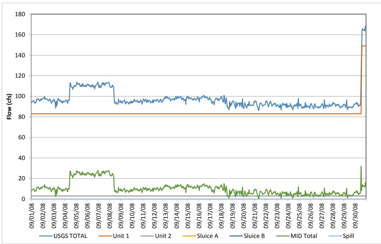
**Figure D-45.** Flow record in September 2008, based on hourly discharges.
