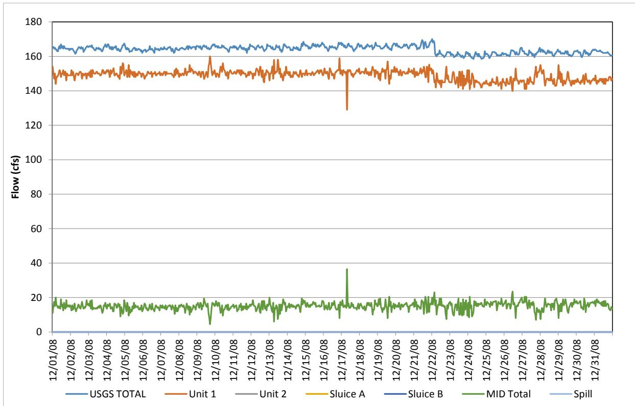
**Figure D-48.** Flow record in December 2008, based on hourly discharges.
