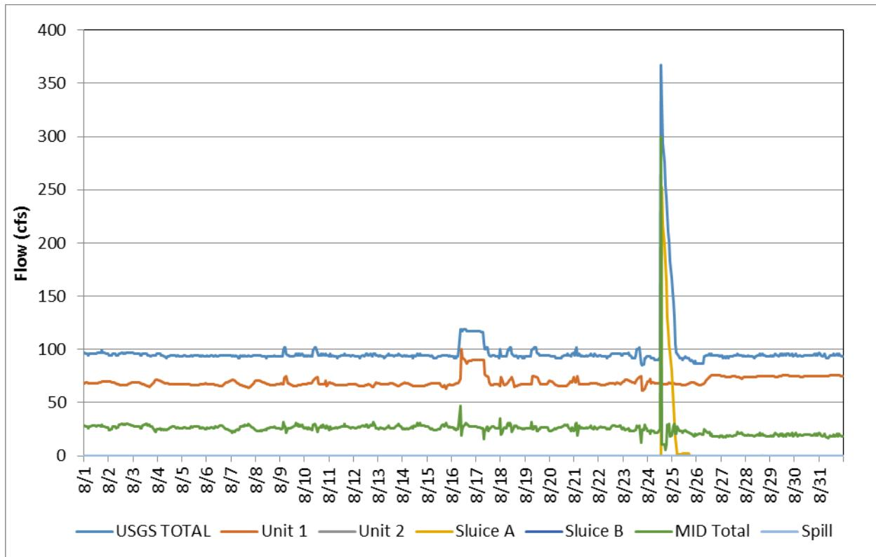
**Figure C-8.** Flow record in August 2016, based on hourly discharges.
