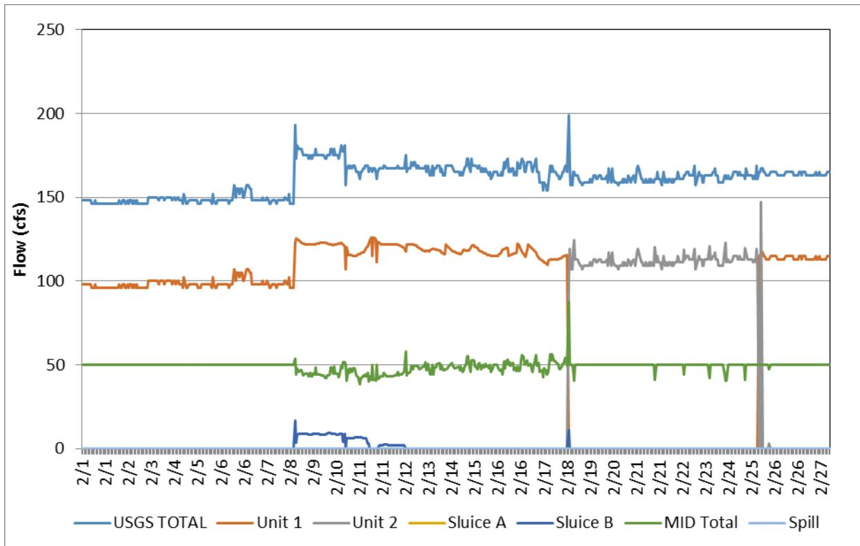
**Figure C-2.** Flow record in February 2016, based on hourly discharges.
