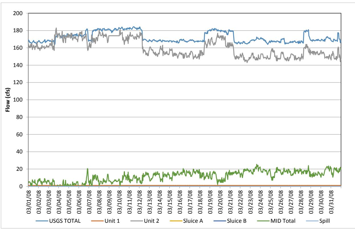
**Figure D-39.** Flow record in March 2008, based on hourly discharges.
