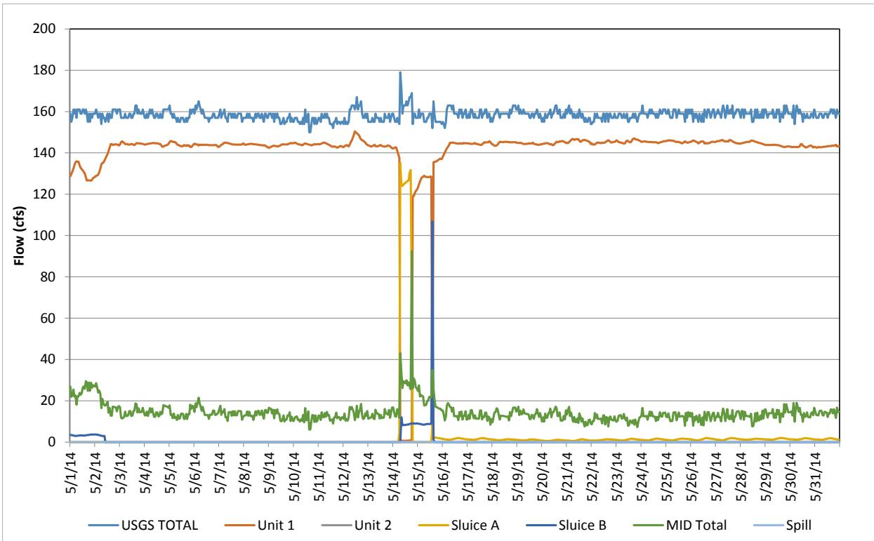
**Figure A-5.** Flow record in May 2014, based on hourly discharges.
