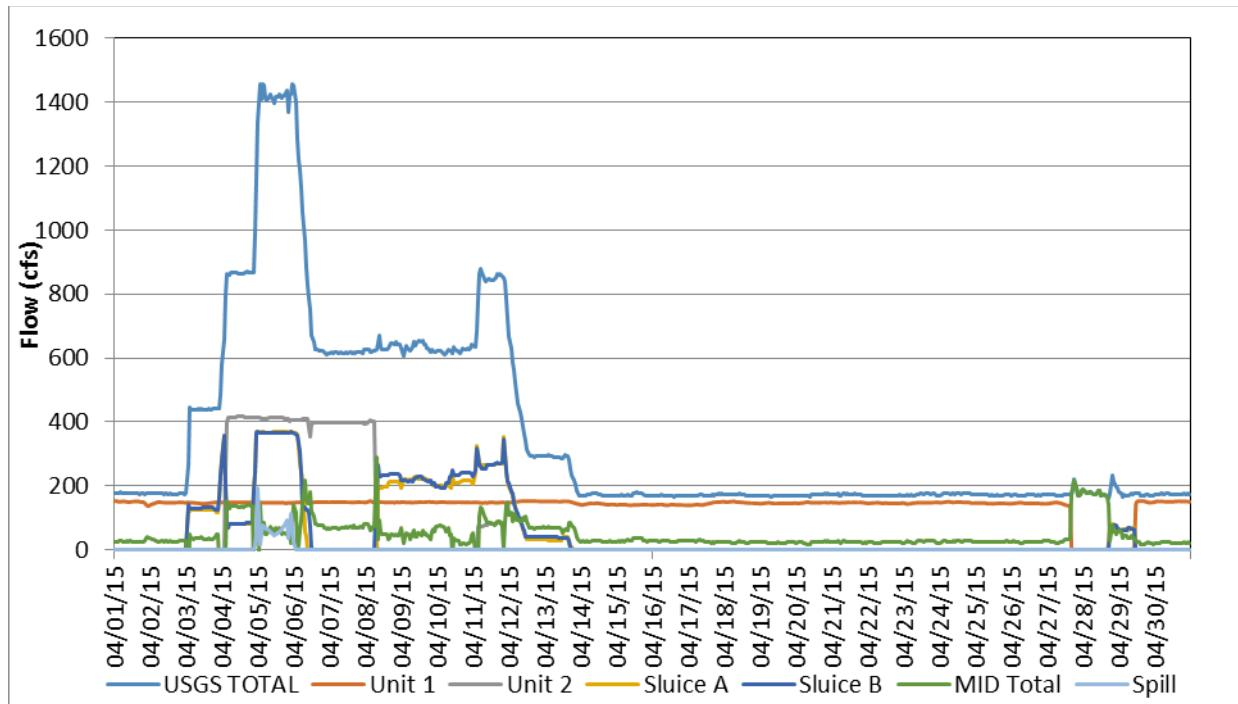
**Figure B-4.** Flow record in April 2015, based on hourly discharges.
