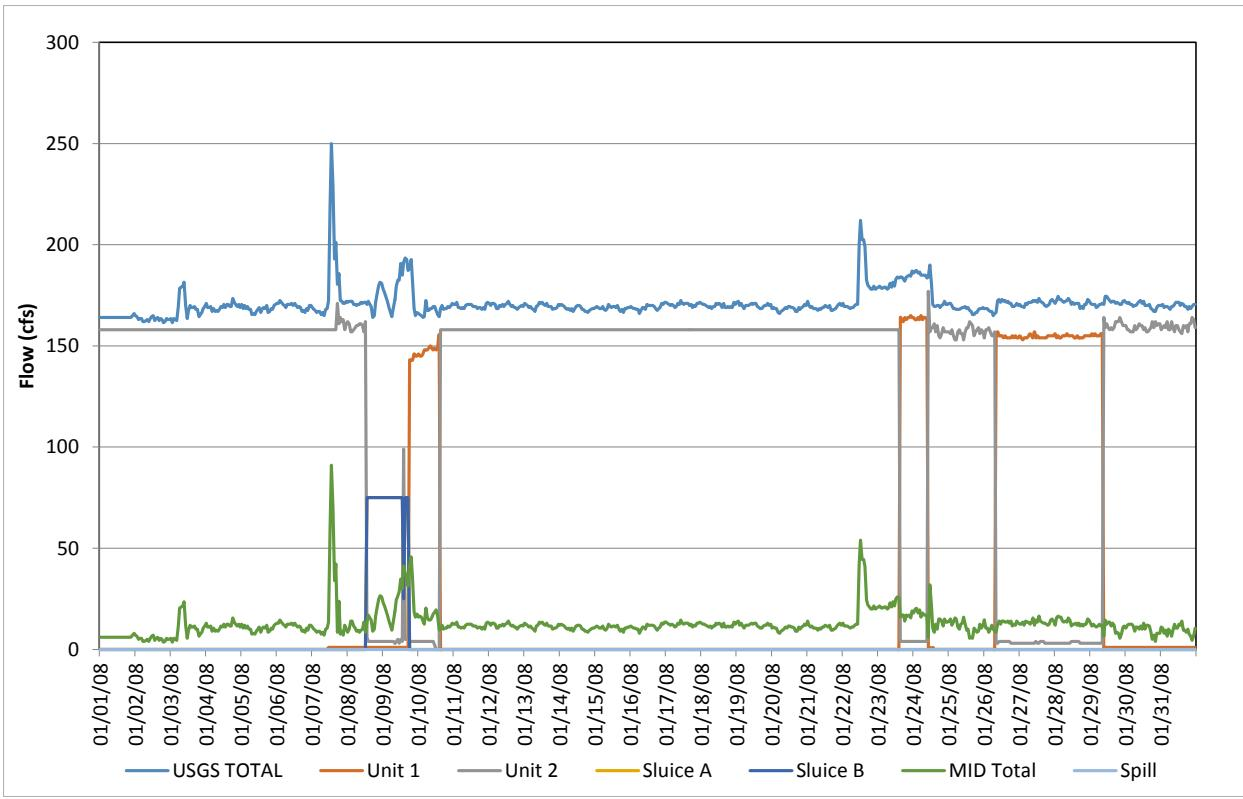
**Figure D-37.** Flow record in January 2008, based on hourly discharges.
