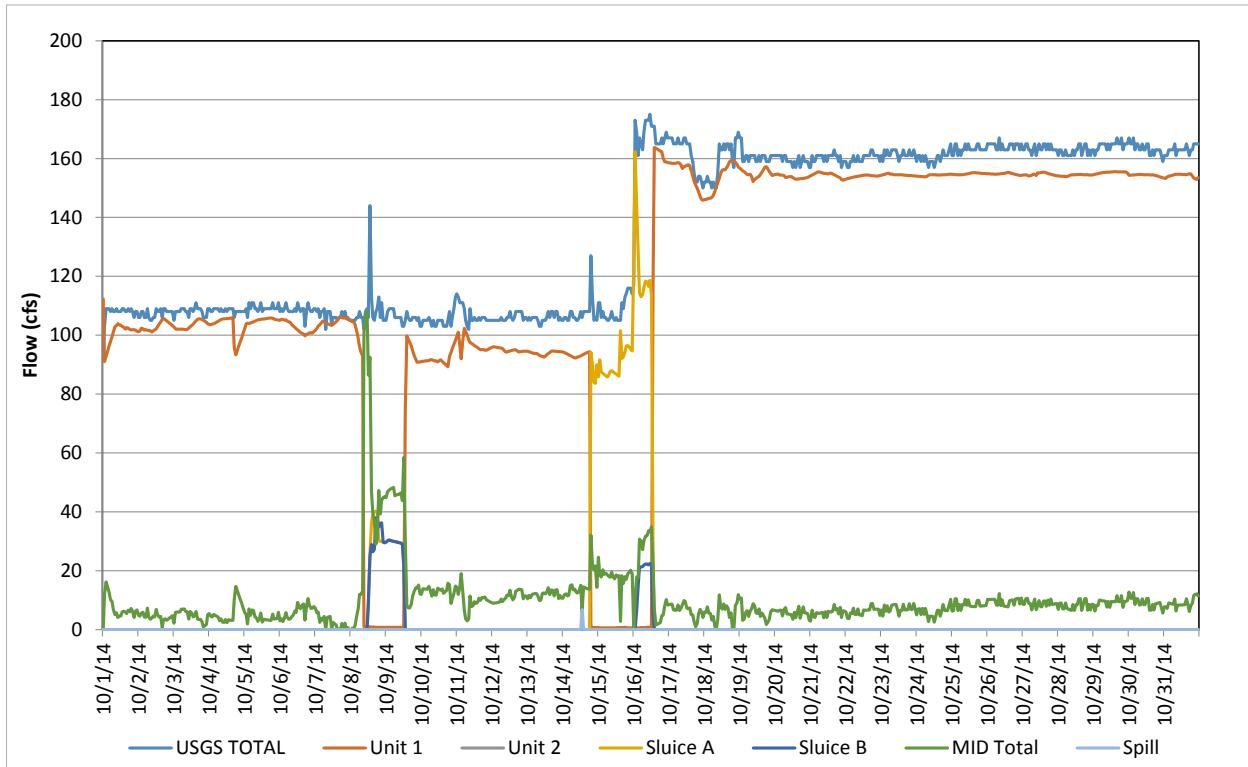
**Figure A-10. Flow record in October 2014, based on hourly discharges.**
