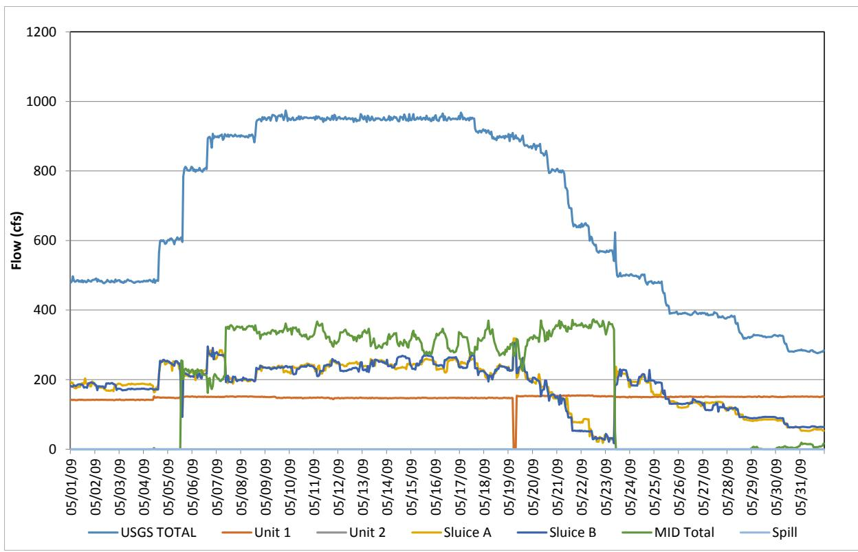
**Figure D-53.** Flow record in May 2009, based on hourly discharges.
