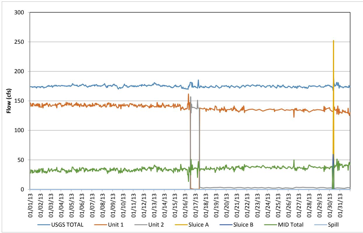
**Figure D-97.** Flow record in January 2013, based on hourly discharges.
