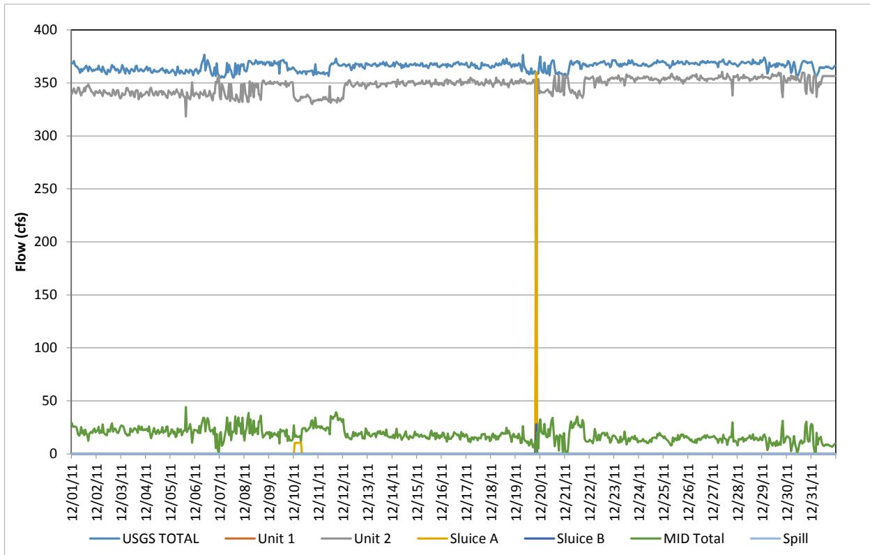
**Figure D-84** Flow record in December 2011, based on hourly discharges.
