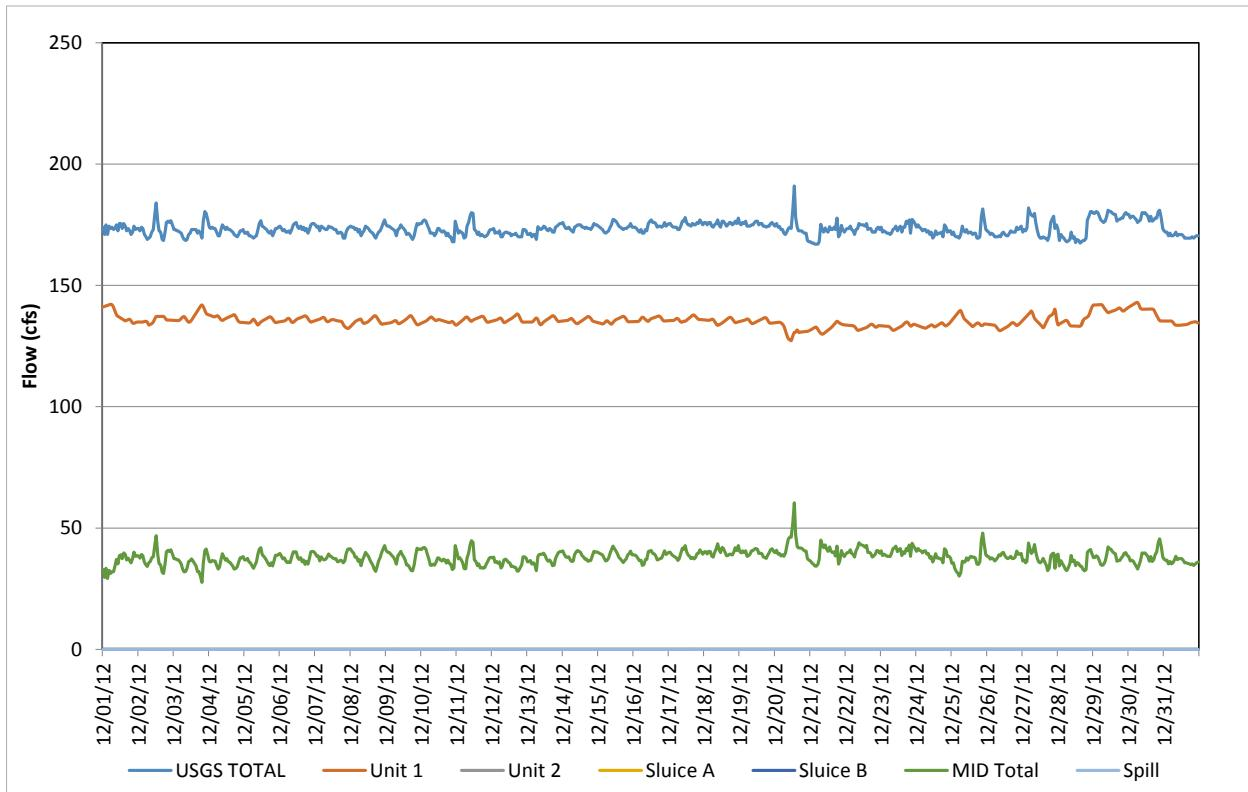
**Figure D-96.** Flow record in December 2012, based on hourly discharges.
