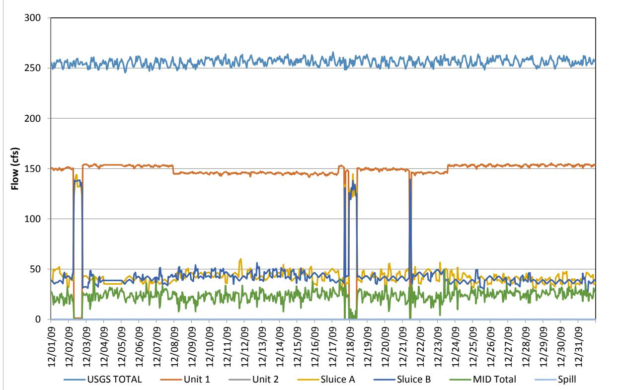
**Figure D-60.** Flow record in December 2009, based on hourly discharges.
