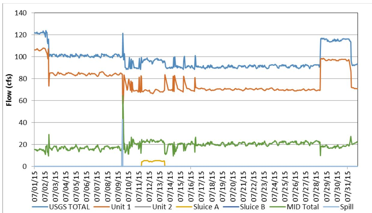
**Figure B-7.** Flow record in July 2015, based on hourly discharges.
