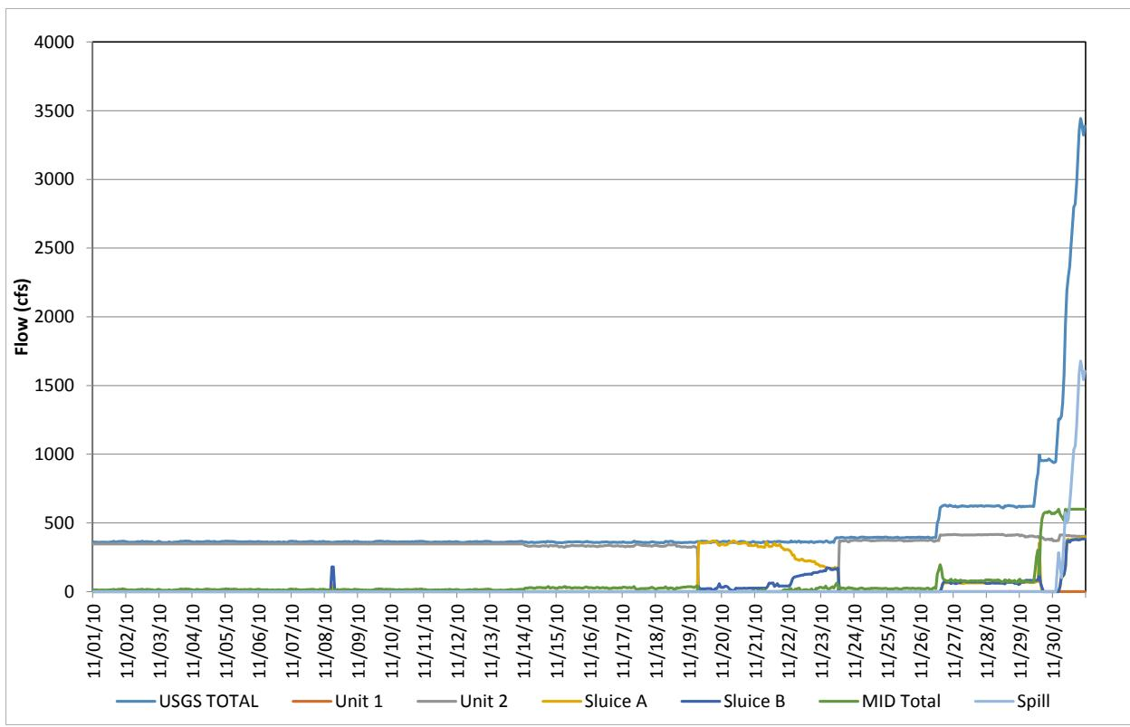
**Figure D-71.** Flow record in November 2010, based on hourly discharges.
