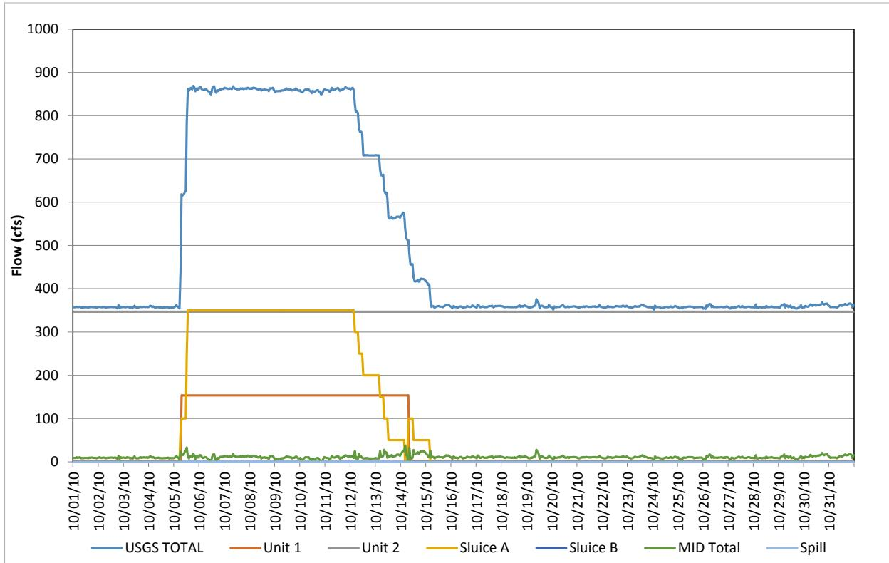
**Figure D-70.** Flow record in October 2010, based on hourly discharges.
