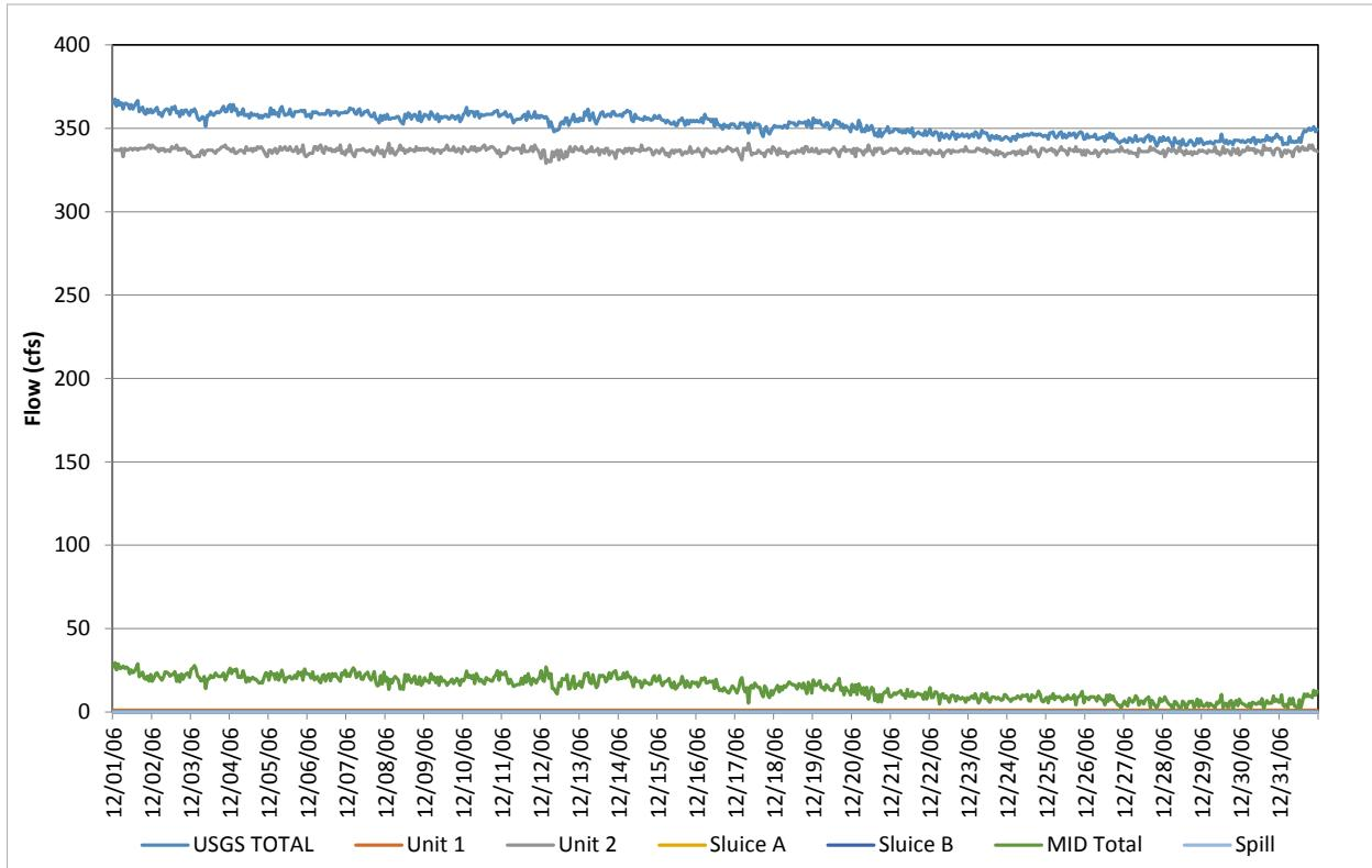
**Figure D-24** Flow record in December 2006, based on hourly discharges.
