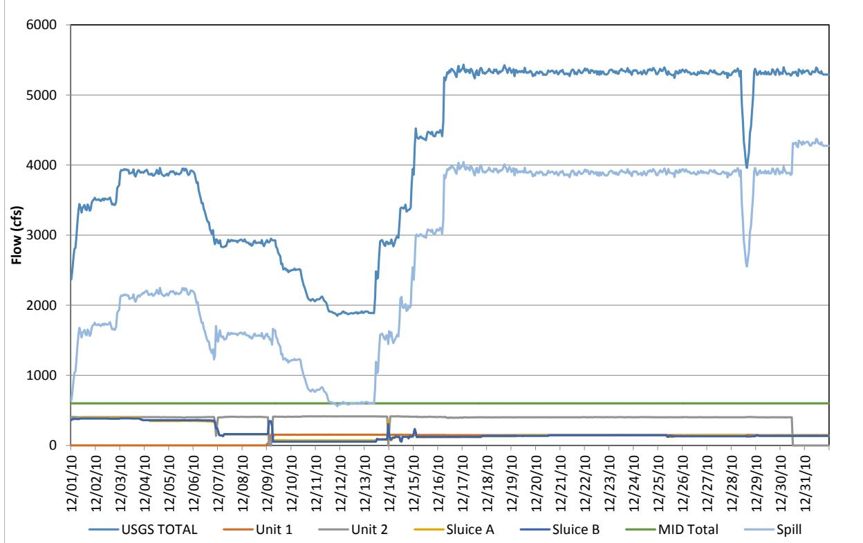
**Figure D-72.** Flow record in December 2010, based on hourly discharges.
