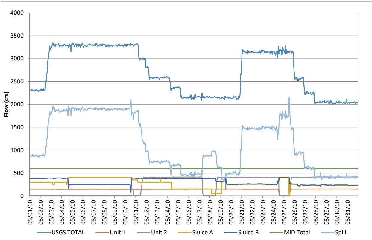
**Figure D-65.** Flow record in May 2010, based on hourly discharges.
