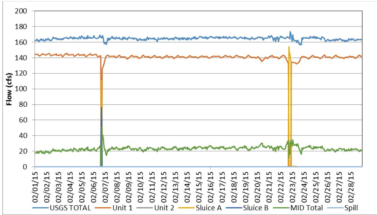
**Figure B-2.** Flow record in February 2015, based on hourly discharges.
