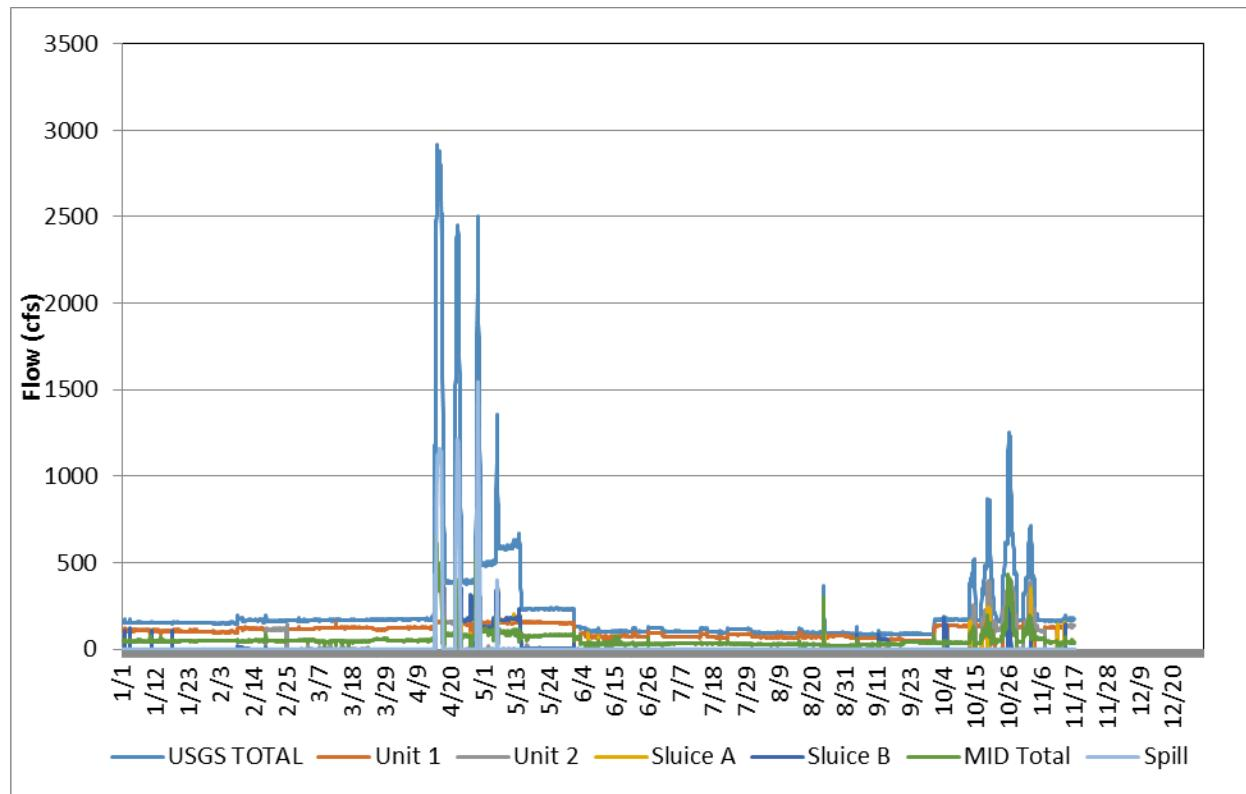
**Figure 3.0-4.** Flow records for year 2016, based on hourly discharges.
