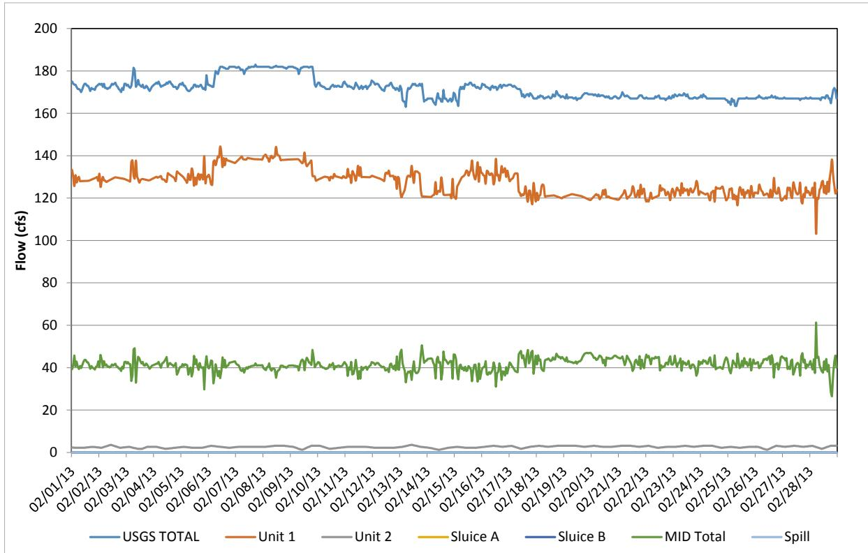
**Figure D-98.** Flow record in February 2013, based on hourly discharges.
