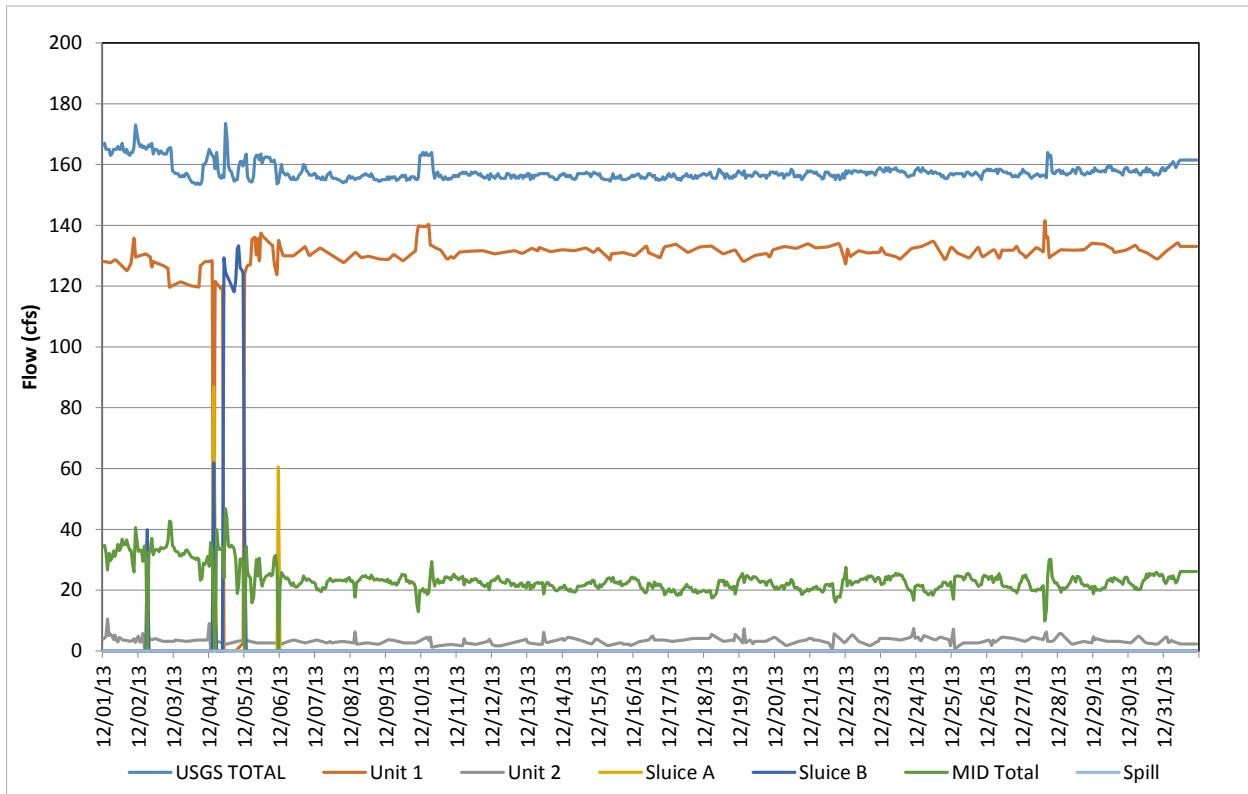
**Figure D-108.** Flow record in December 2013, based on hourly discharges.
