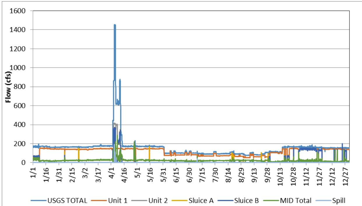
**Figure 3.0-3.** Flow records for year 2015, based on hourly discharges.
