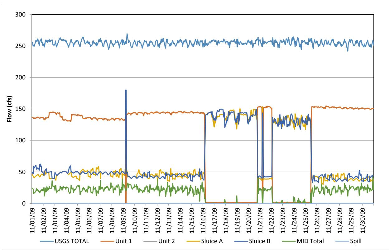
**Figure D-59.** Flow record in November 2009, based on hourly discharges.
