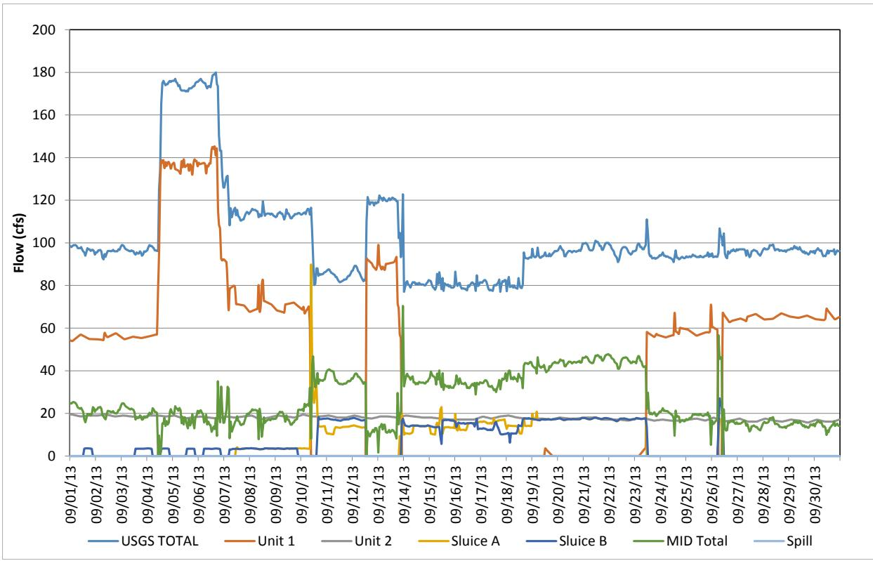
**Figure D-105.** Flow record in September 2013, based on hourly discharges.
