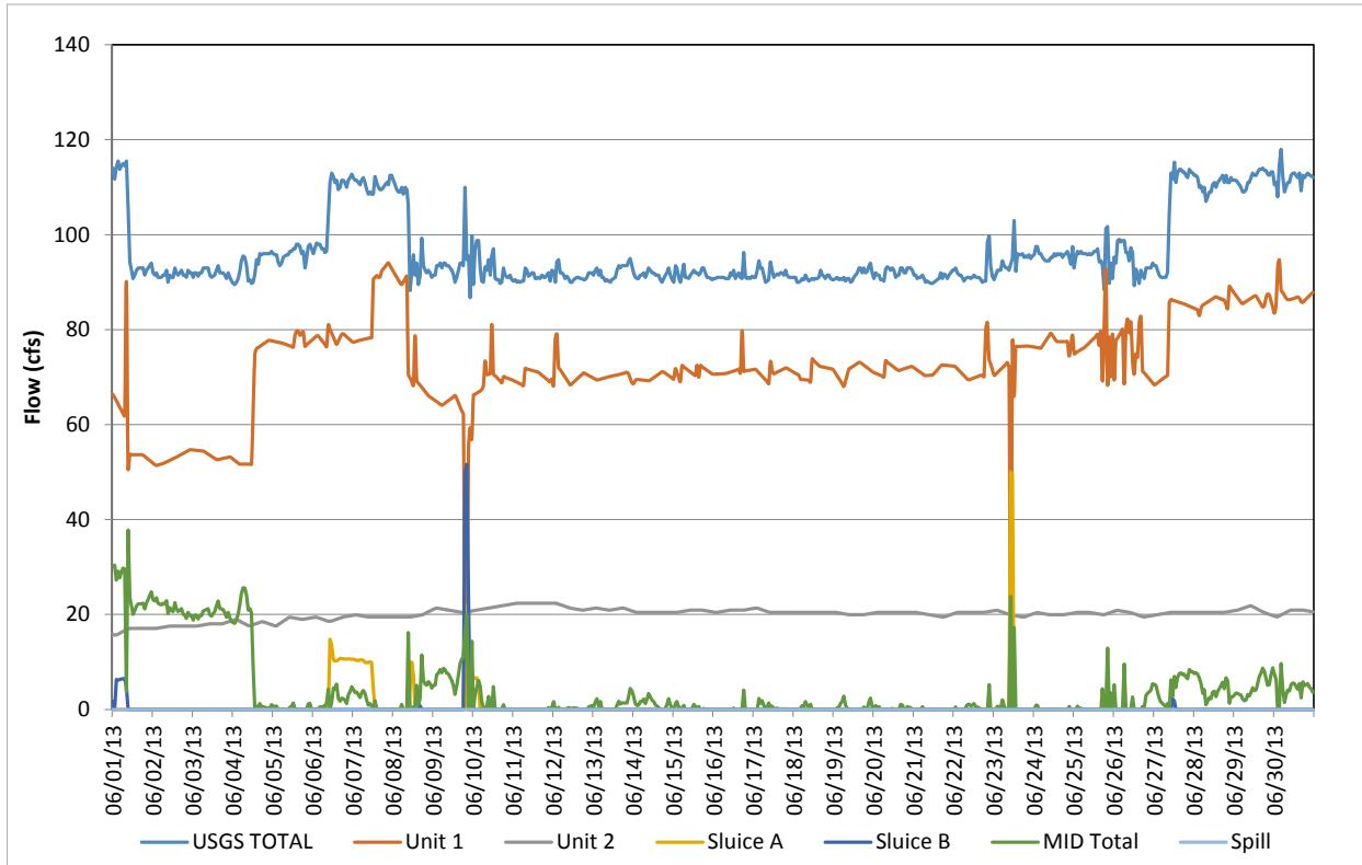
**Figure D-102.** Flow record in June 2013, based on hourly discharges.
