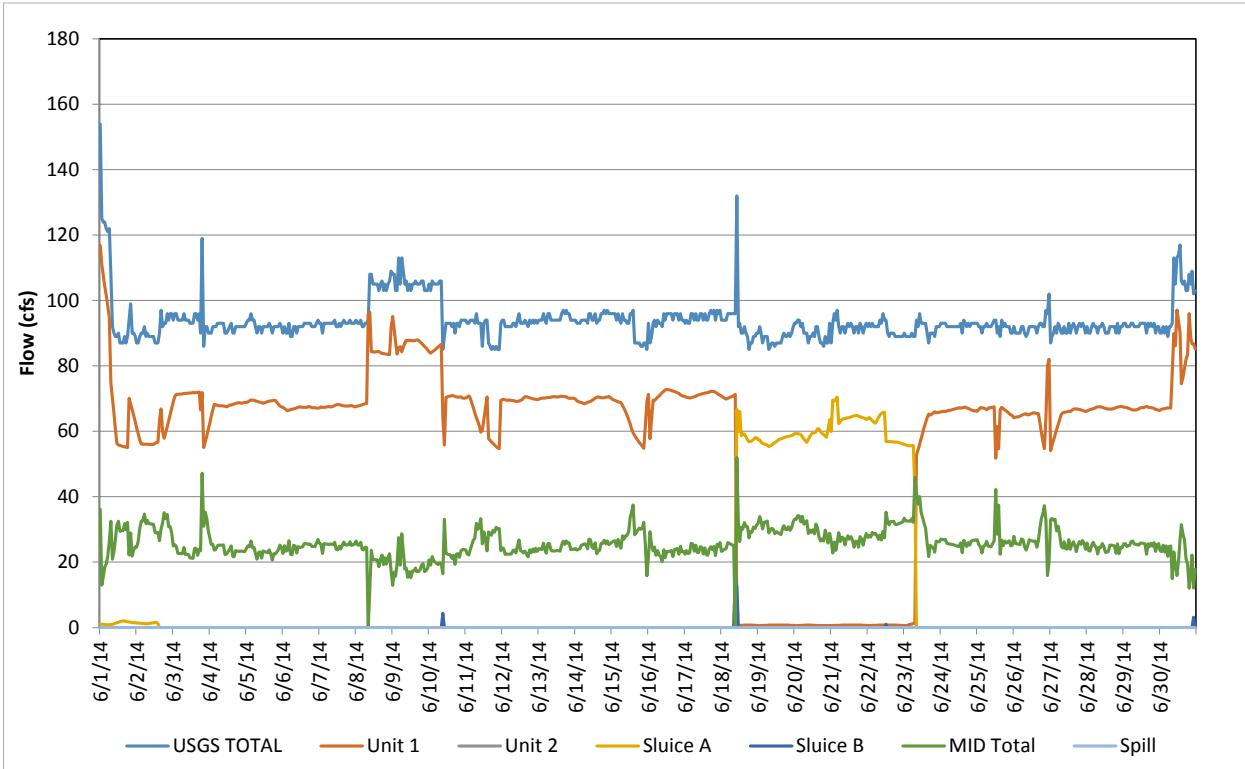
**Figure A-6.** Flow record in June 2014, based on hourly discharges.
