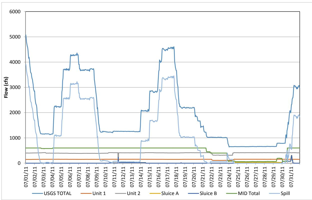
**Figure D-79.** Flow record in July 2011, based on hourly discharges.
