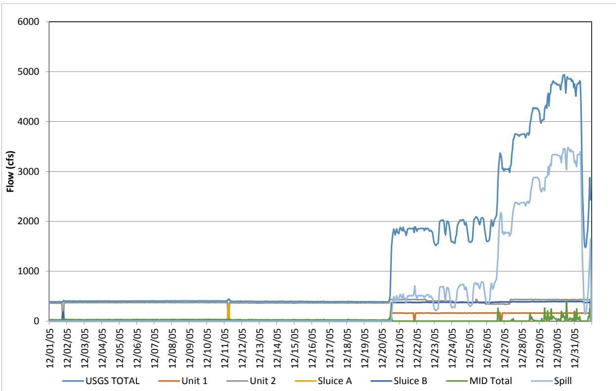
**Figure D-12.** Flow record in December 2005, based on hourly discharges.
