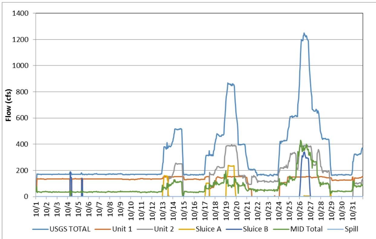
**Figure C-10.** Flow record in October 2016, based on hourly discharges.
