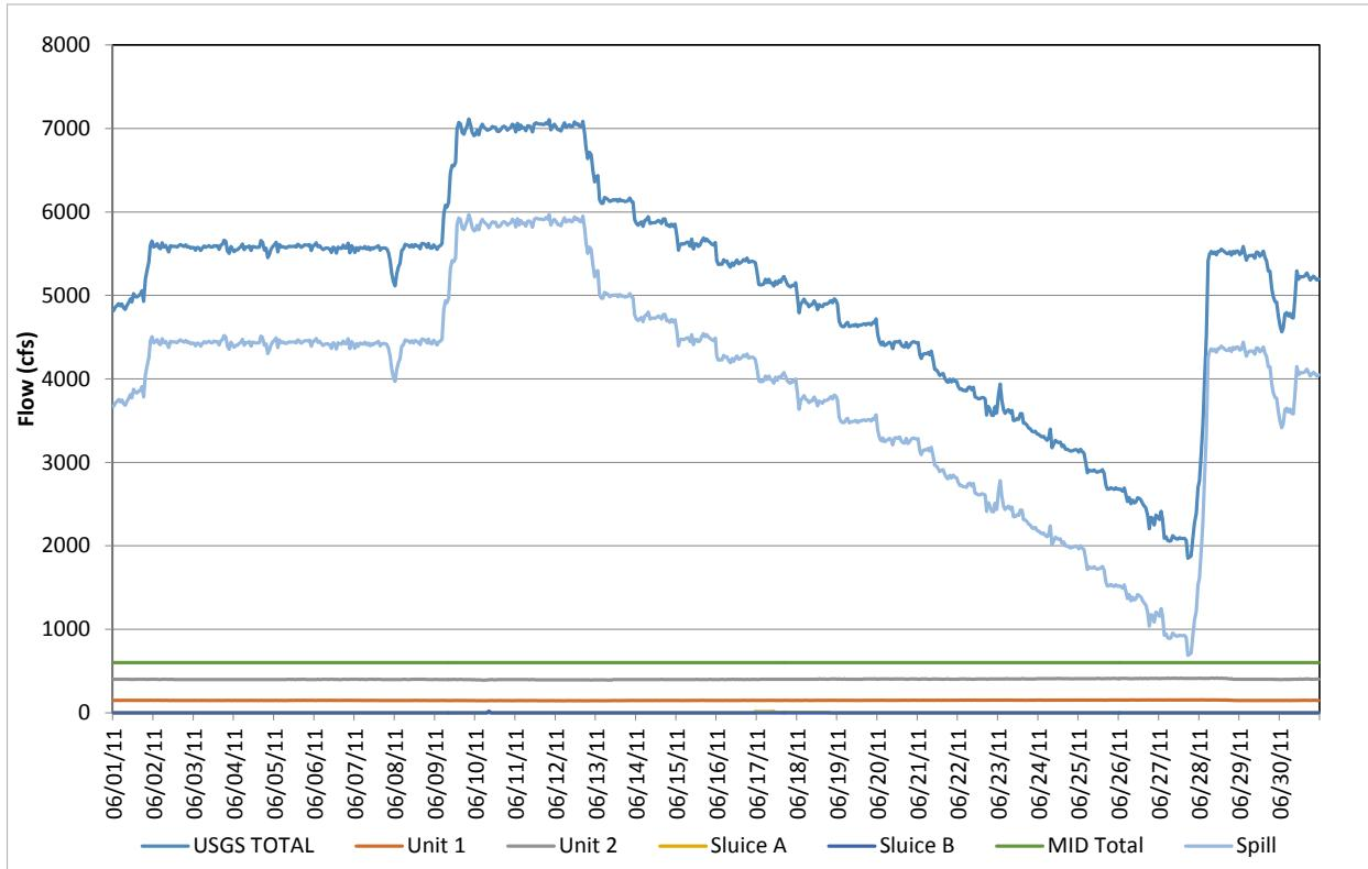
**Figure D-78.** Flow record in June 2011, based on hourly discharges.
