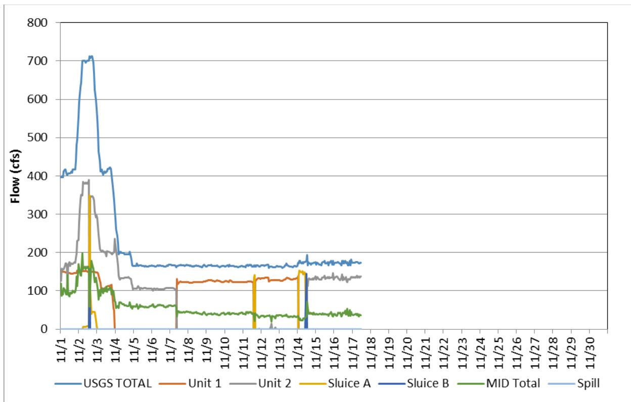
**Figure C-11.** Flow record in November 2016, based on hourly discharges.
