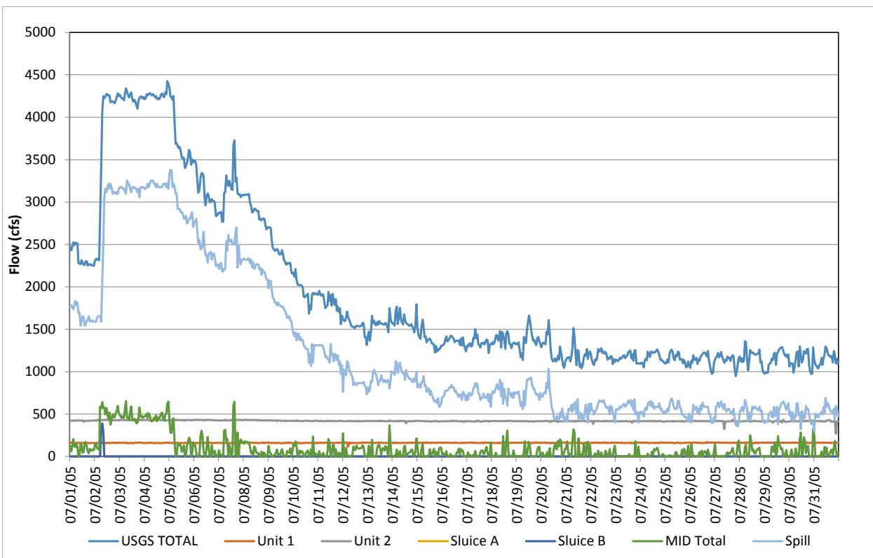
**Figure D-7.** Flow record in July 2005, based on hourly discharges.
