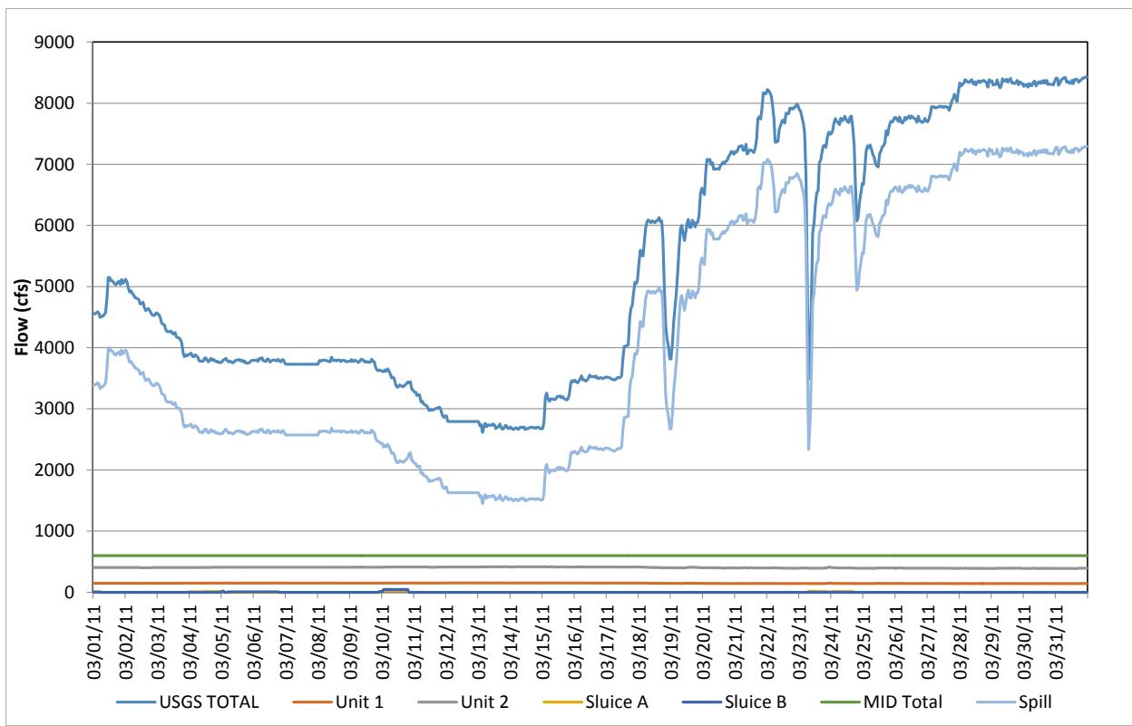
**Figure D-75.** Flow record in March 2011, based on hourly discharges.
