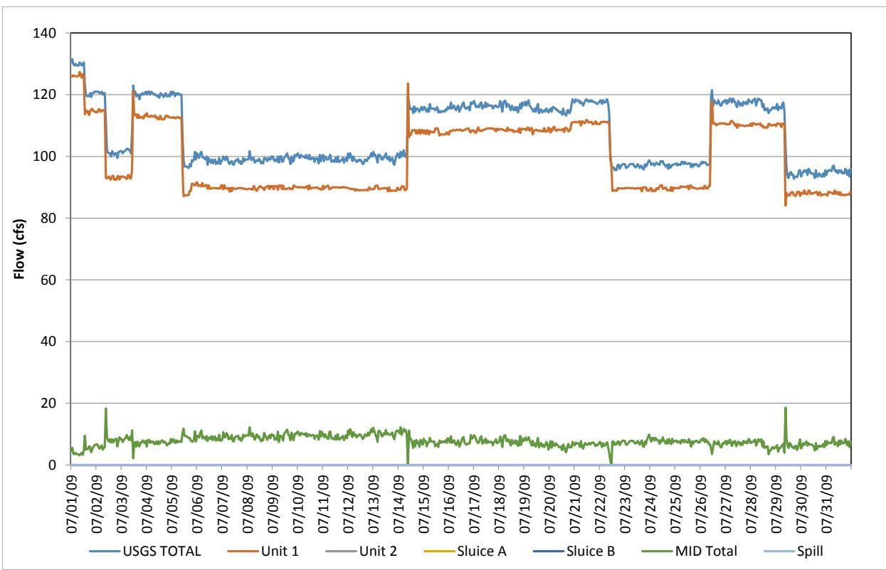
**Figure D-55.** Flow record in July 2009, based on hourly discharges.
