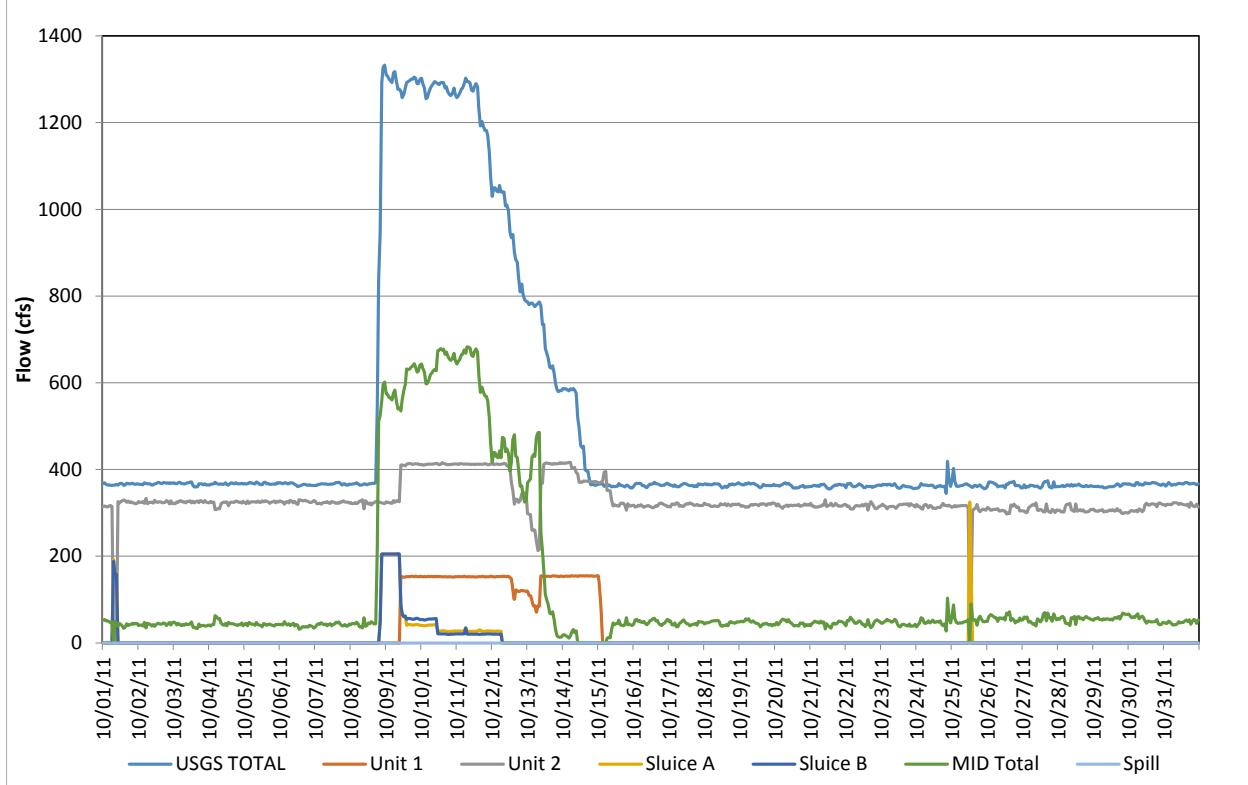
**Figure D-82.** Flow record in October 2011, based on hourly discharges.
