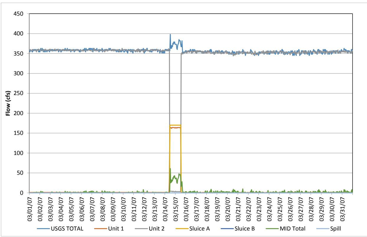
**Figure D-27.** Flow record in March 2007, based on hourly discharges.
