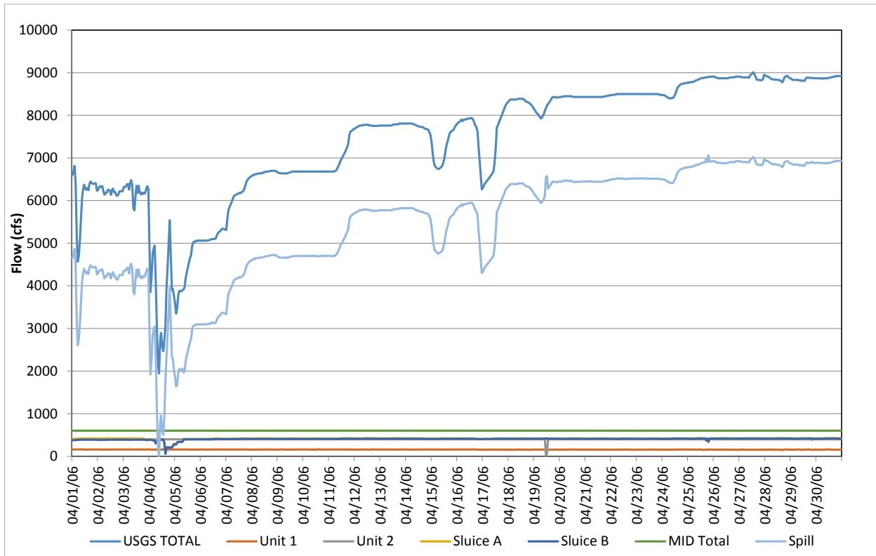
**Figure D-16.** Flow record in April 2006, based on hourly discharges.
