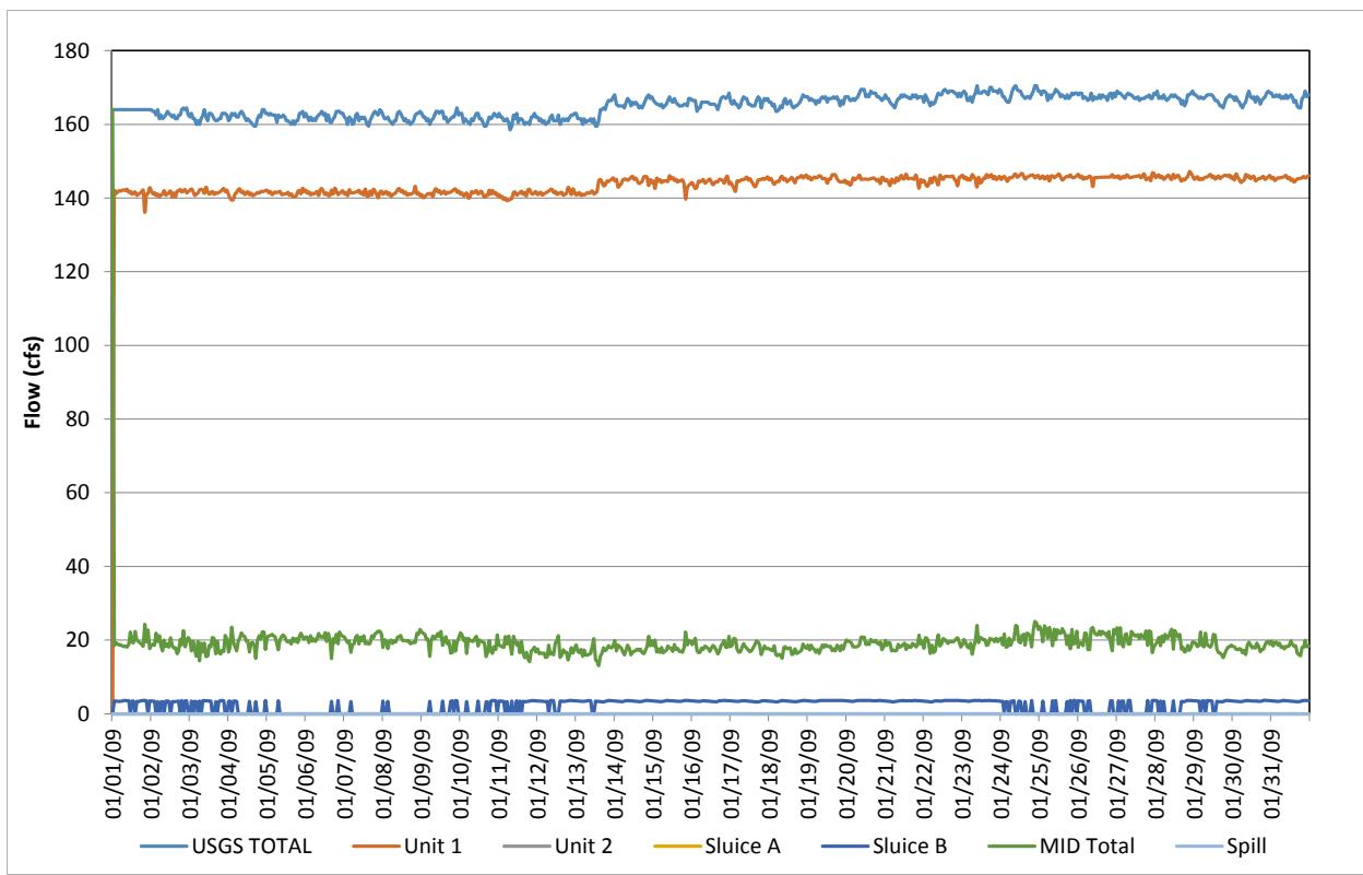
**Figure D-49.** Flow record in January 2009, based on hourly discharges.
