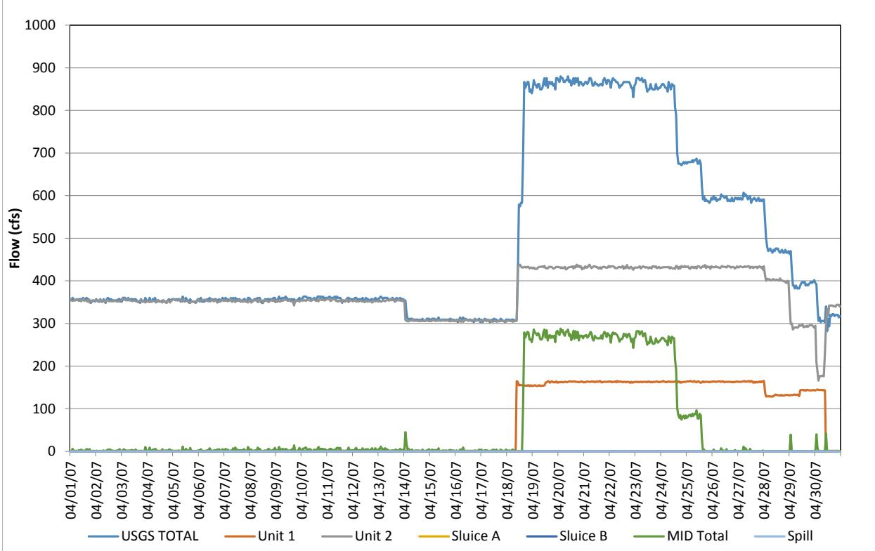
**Figure D-27.** Flow record in April 2007, based on hourly discharges.
