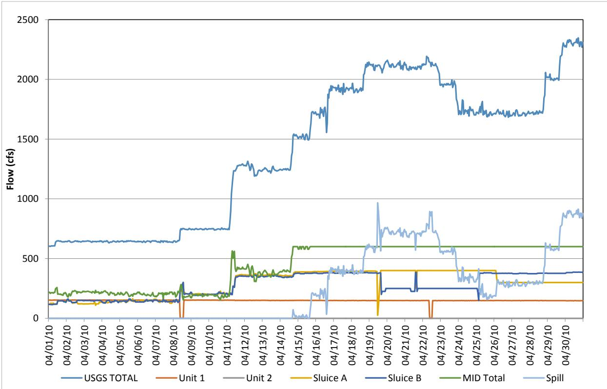
**Figure D-64.** Flow record in April 2010, based on hourly discharges.
