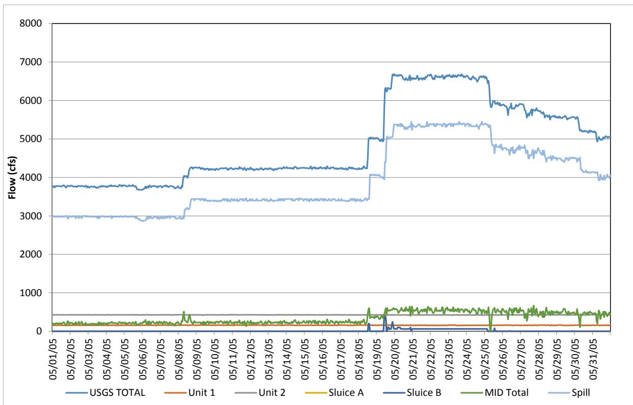
**Figure D-5.** Flow record in May 2005, based on hourly discharges.
