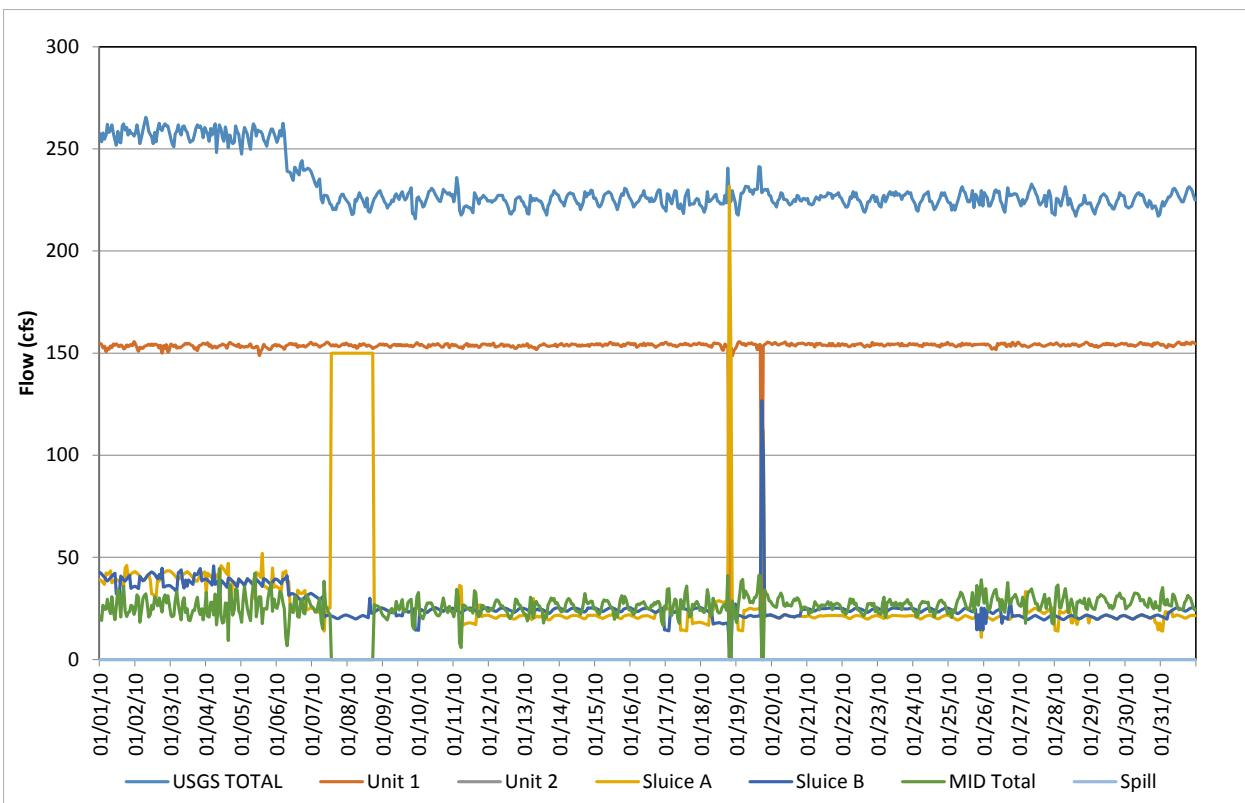
**Figure D-61.** Flow record in January 2010, based on hourly discharges.
