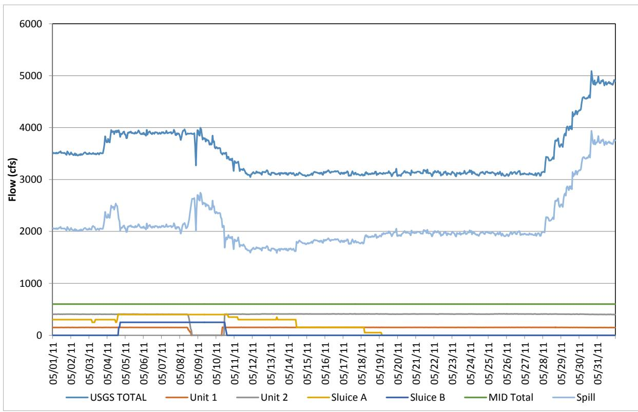
**Figure D-77.** Flow record in May 2011, based on hourly discharges.
