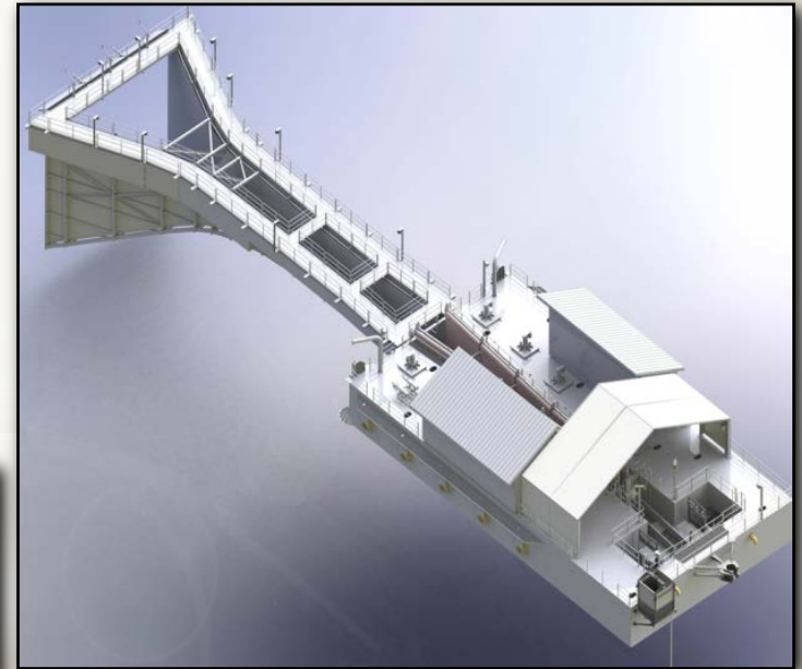
Cushman Surface Collector and Fish Handling Equipment. Figures by Tacoma Power
