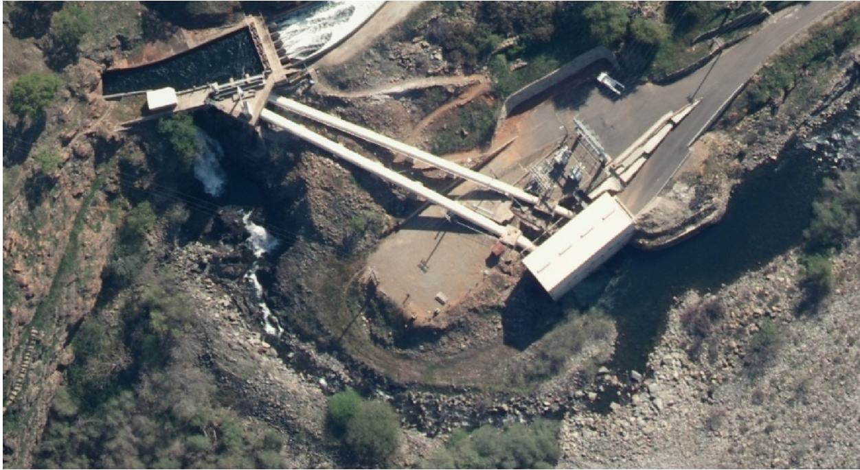
Figure 3.5-6. Aerial photo of sluice gate channel area, forebay, penstock intakes, powerhouse and upper end of tailrace channel.
