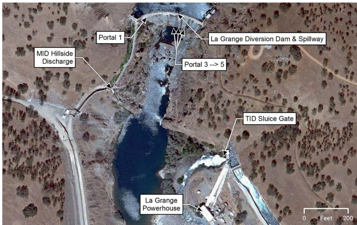
**Figure 2.0-1. Location of five discharge structures at the La Grange Project.**
