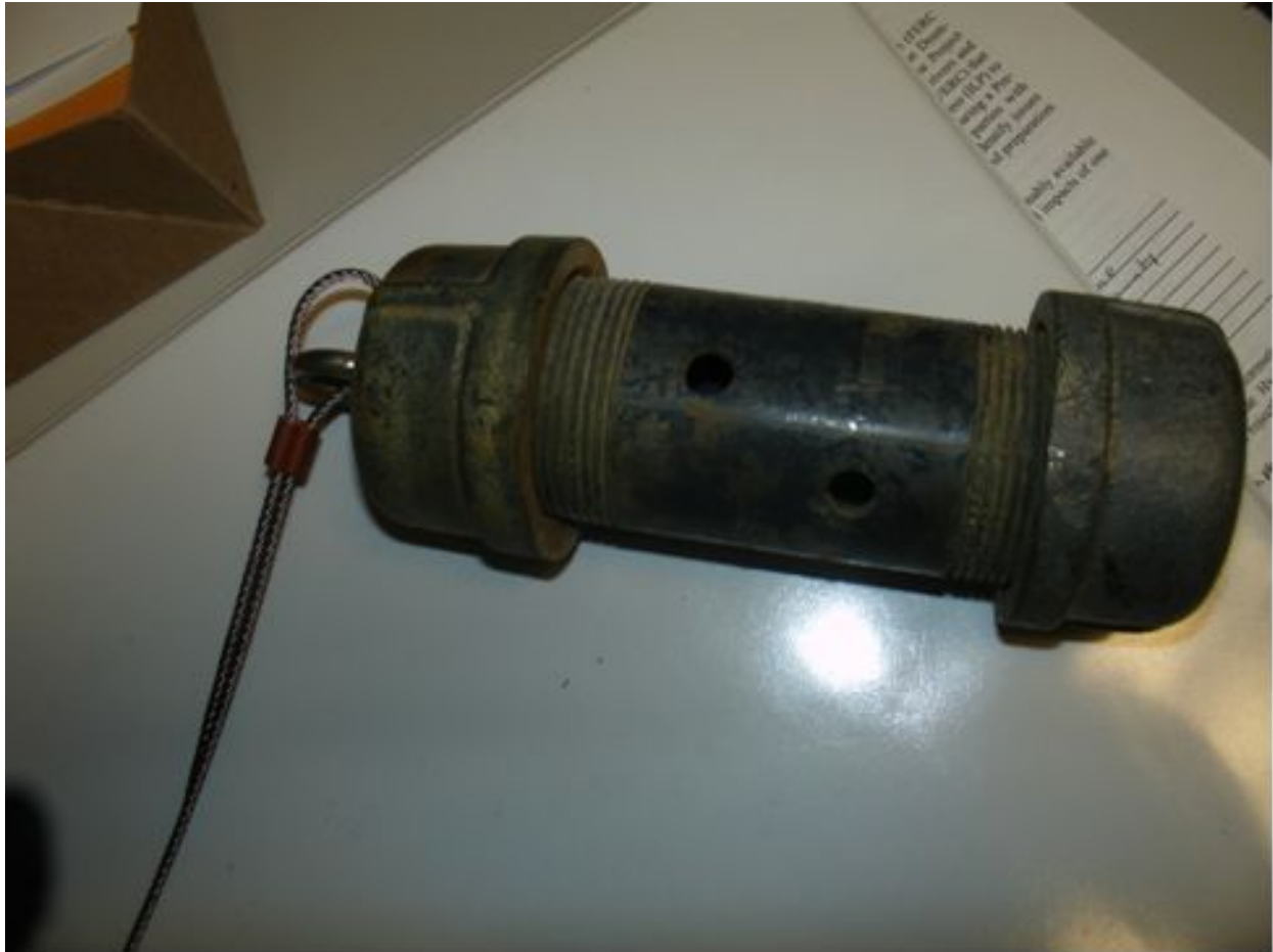
Figure A-1. Photograph of normal water temperature recorder housing. Approximate size is 4-6 inches with 2-8 feet of associated cabling.
