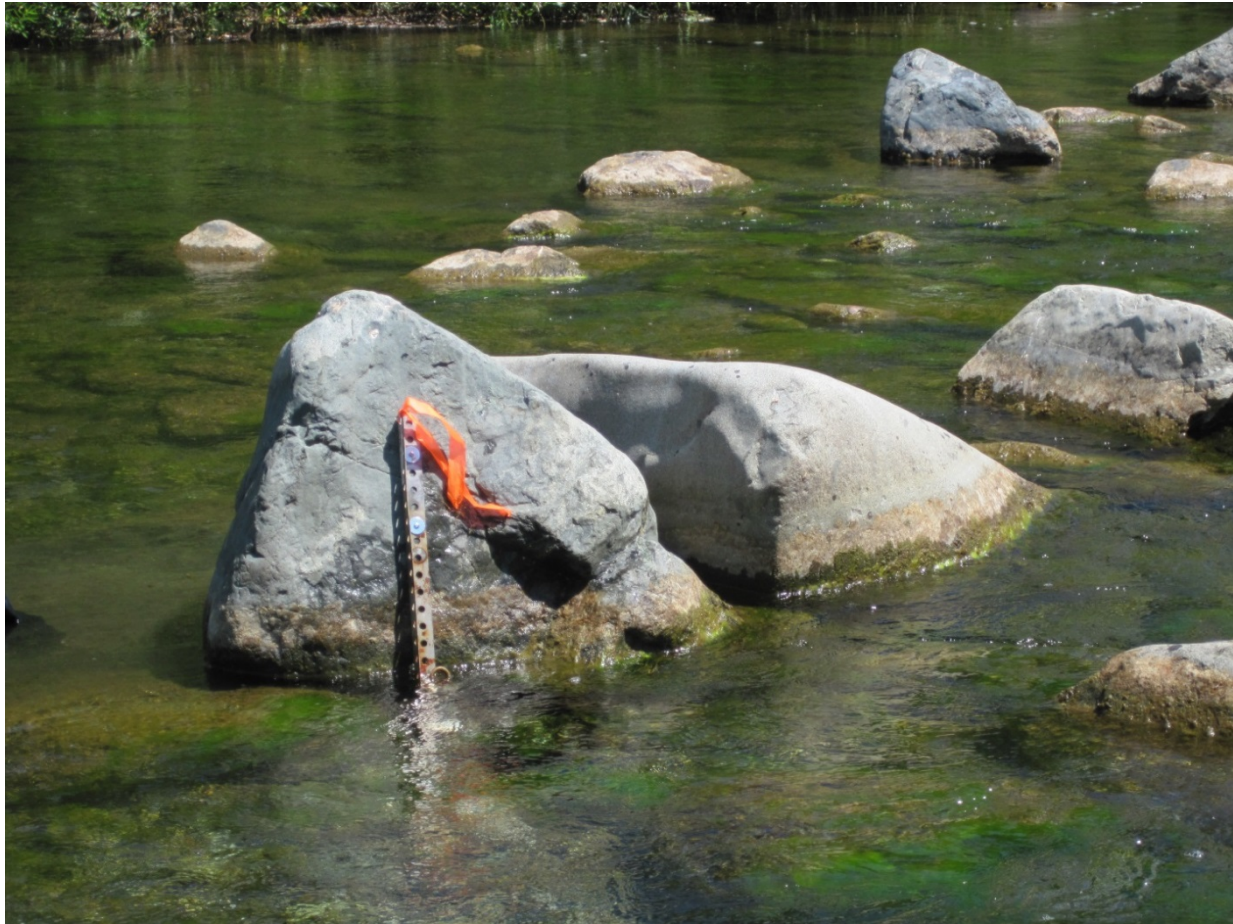
Figure A-2. Example of level logger installation. Bolted (removable) to boulder or bedrock.
