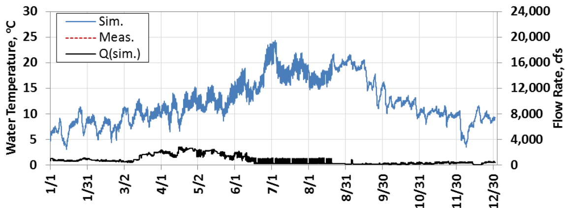
Figure F-43. Comparison of measured (Meas.) and simulated (Sim.) water temperature above North Fork Tuolumne River confluence for the calibration year 2013. Flow rate (in cfs) is presented in the secondary axis. (Note: Measured data for this location not available during this period.)
