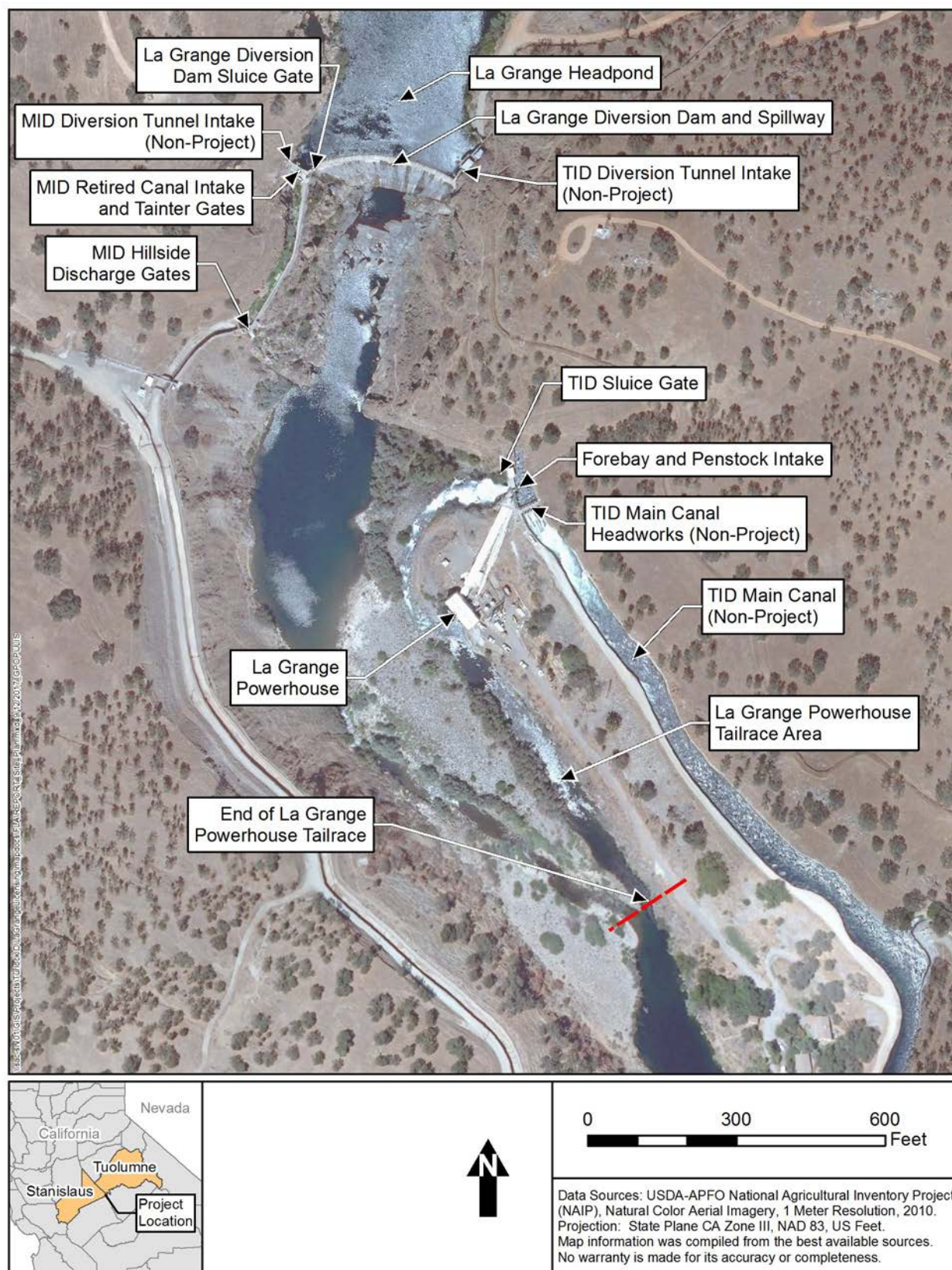
Figure 1.1-2. La Grange Hydroelectric Project site plan.
