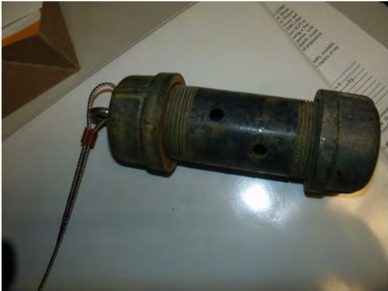
Figure 1. Photograph of normal water temperature recorder housing. Approximate size is 4-6 inches with 2-8 feet of associated cabling.
