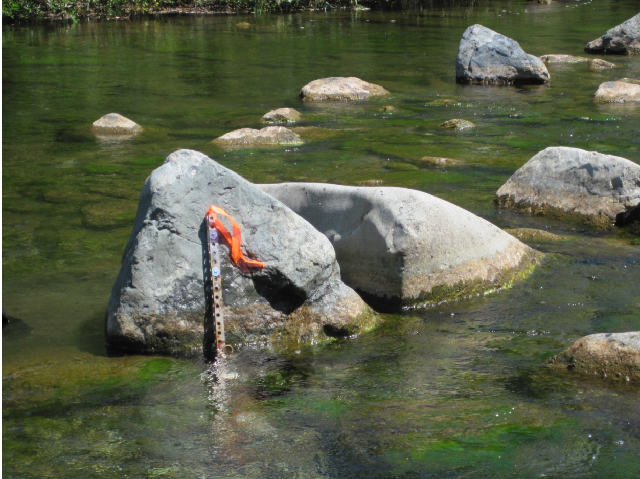
Figure 2. Example of level logger installation. Bolted (removable) to boulder or bedrock.
