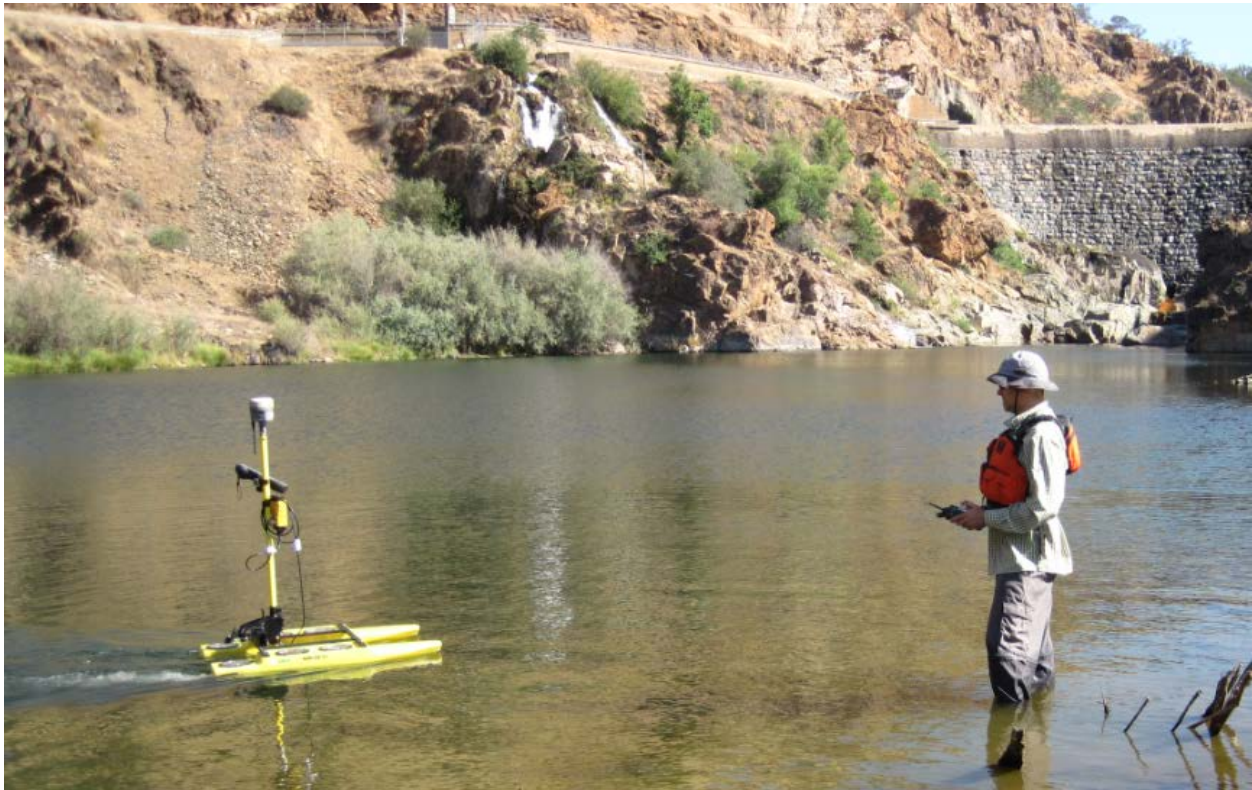
Figure 4.1-2. Bathymetric survey of plunge pool below La Grange Diversion Dam.
