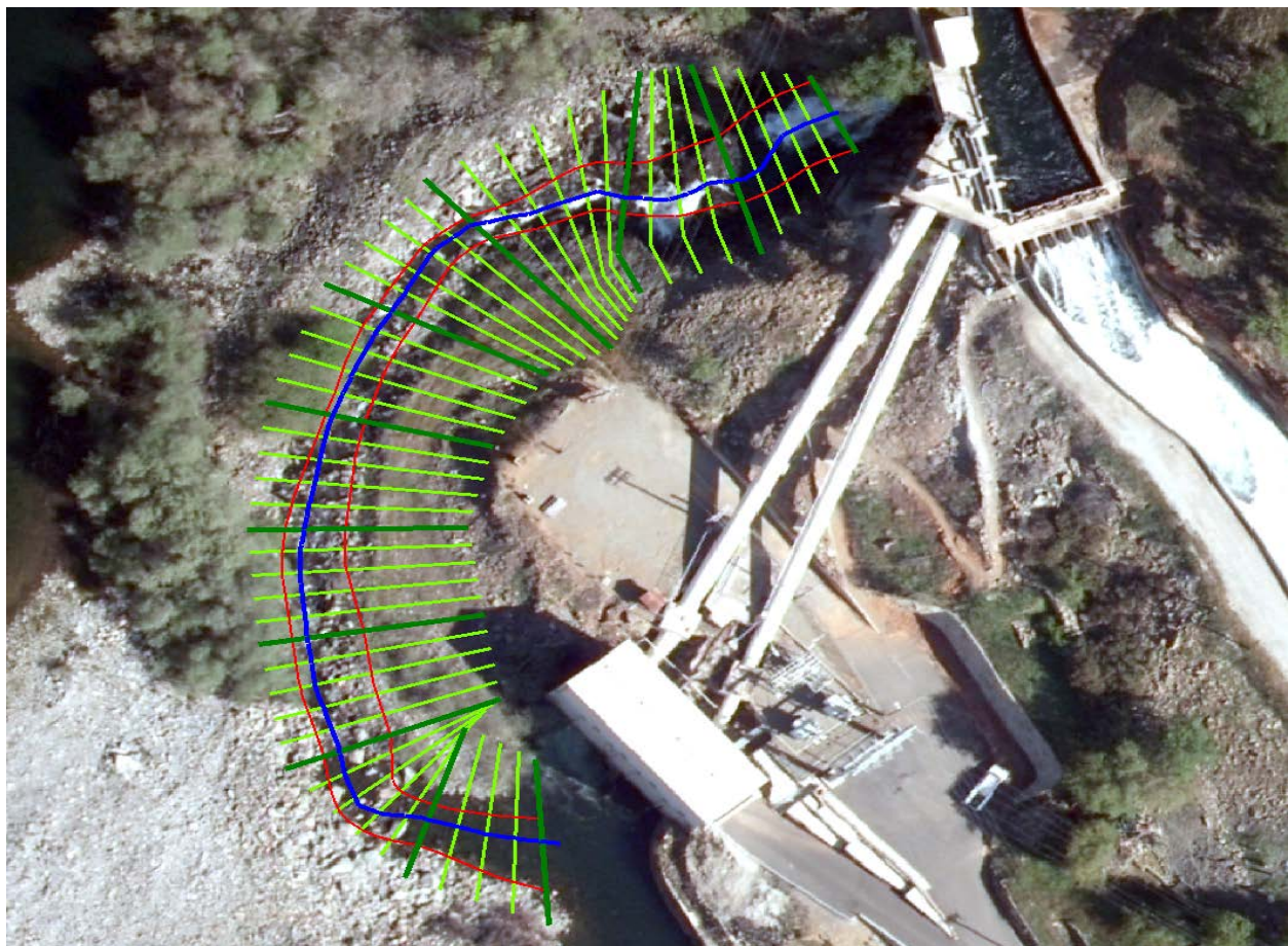
Figure B-3. HEC-RAS model geometry superimposed on aerial photo.
