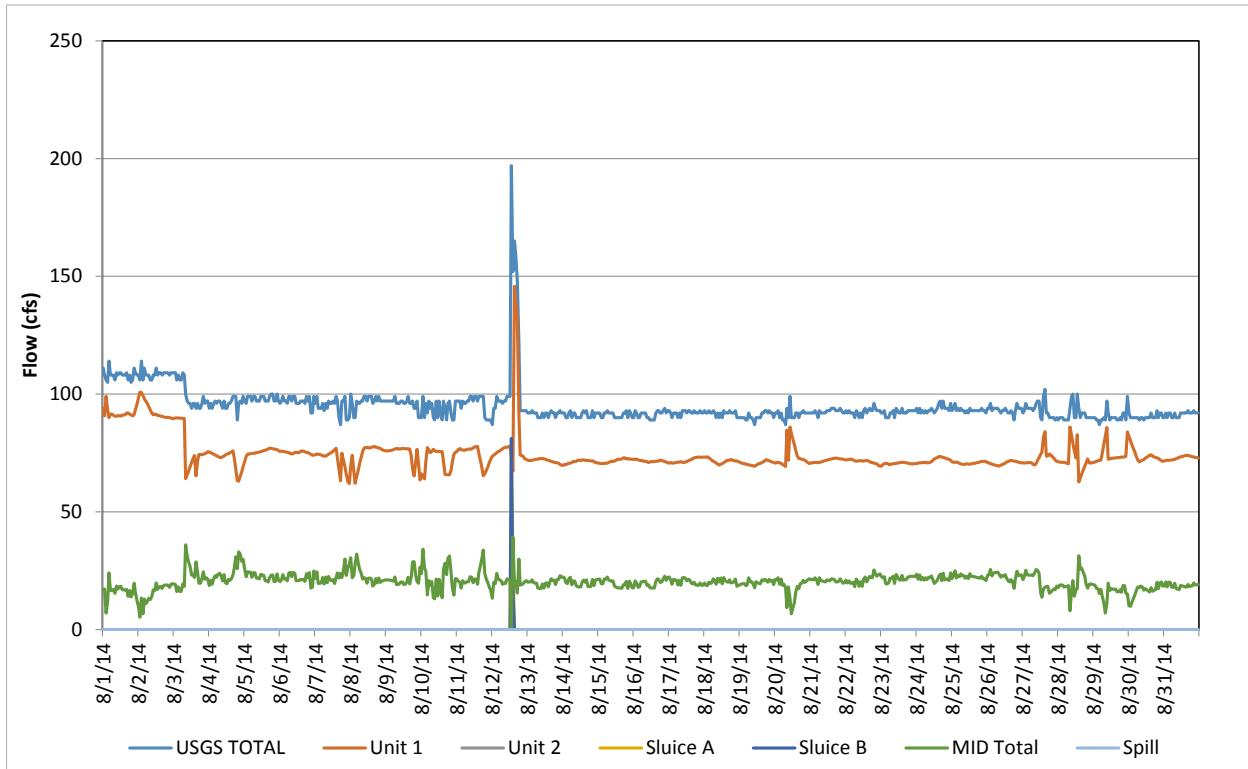
**Figure A-8. Flow record in August 2014, based on hourly discharges.**
