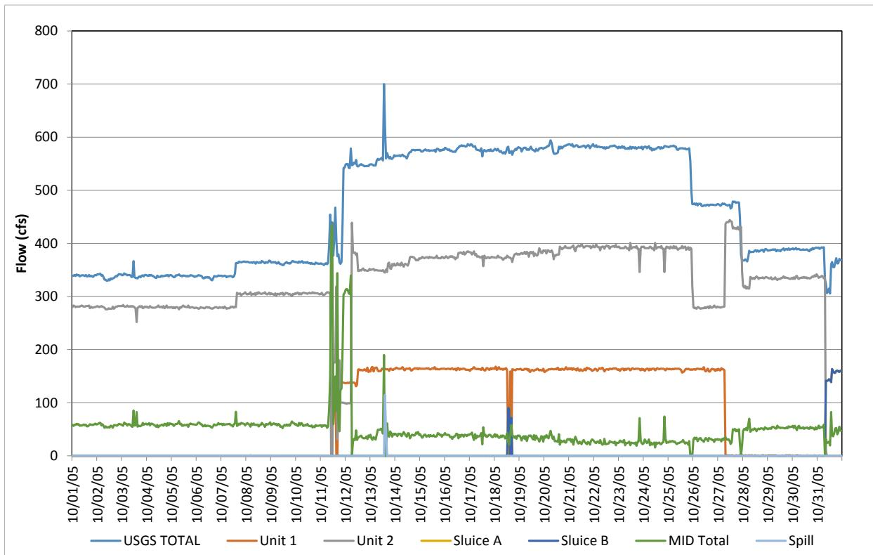
**Figure D-10.** Flow record in October 2005, based on hourly discharges.
