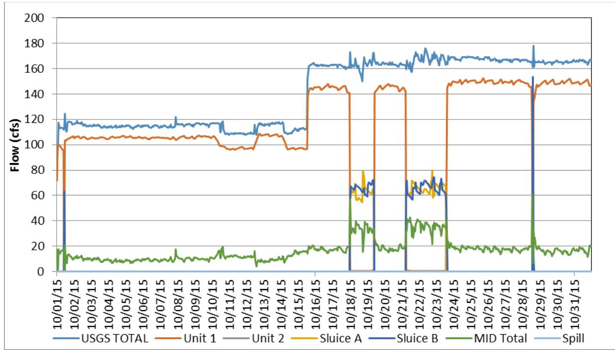
**Figure B-10.** Flow record in October 2015, based on hourly discharges.
