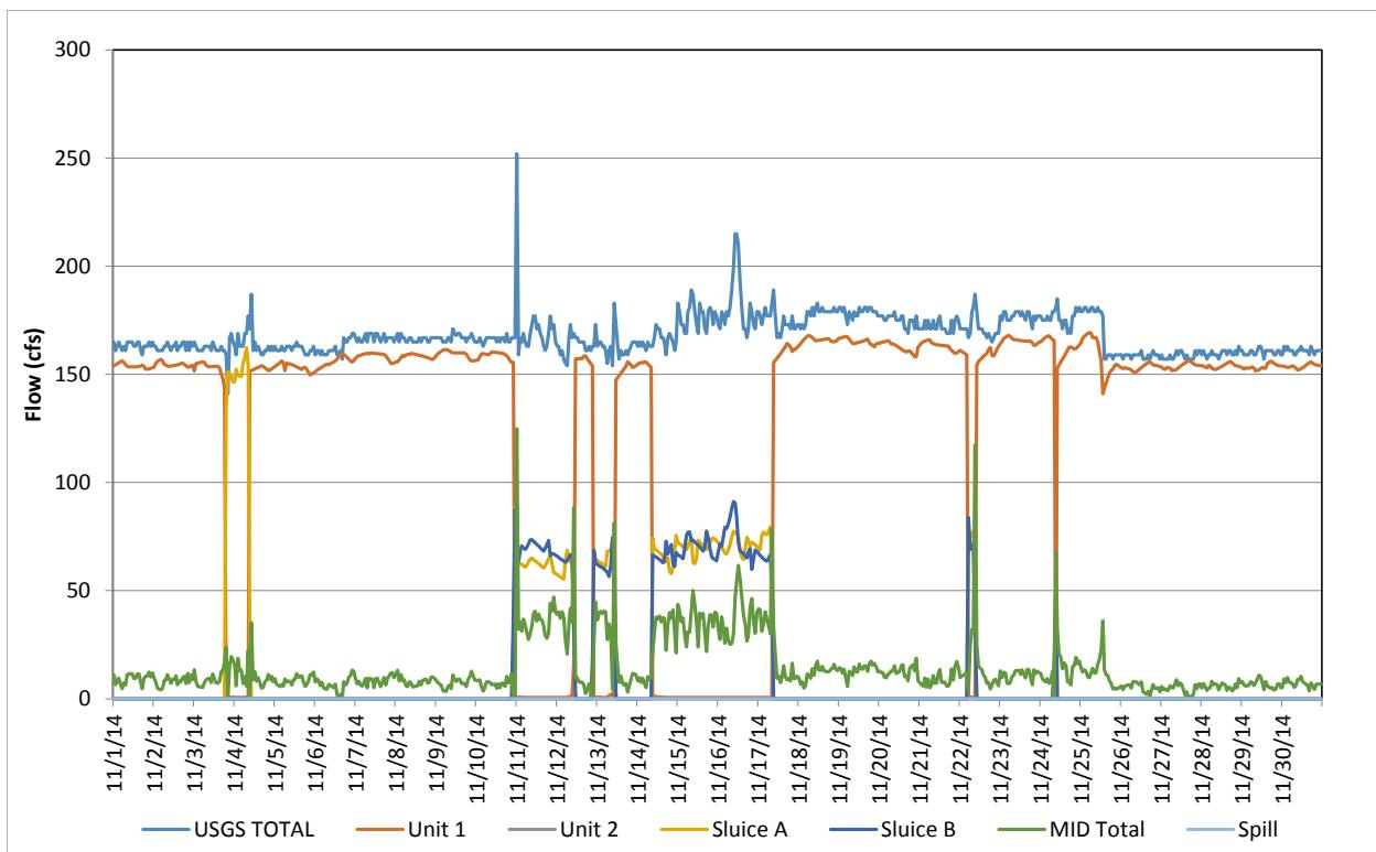
**Figure A-11.** Flow record in November 2014, based on hourly discharges.
