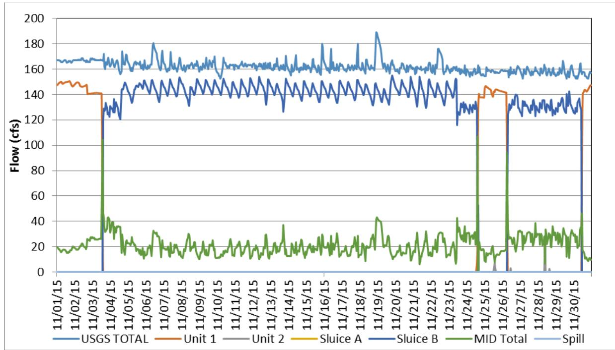
**Figure B-11.** Flow record in November 2015, based on hourly discharges.
