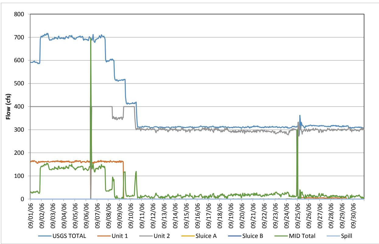
**Figure D-21.** Flow record in September 2006, based on hourly discharges.
