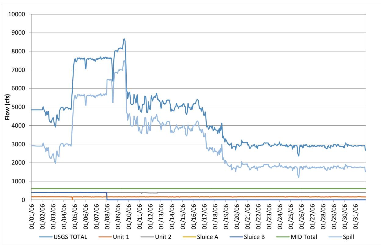
**Figure D-13.** Flow record in January 2006, based on hourly discharges.
