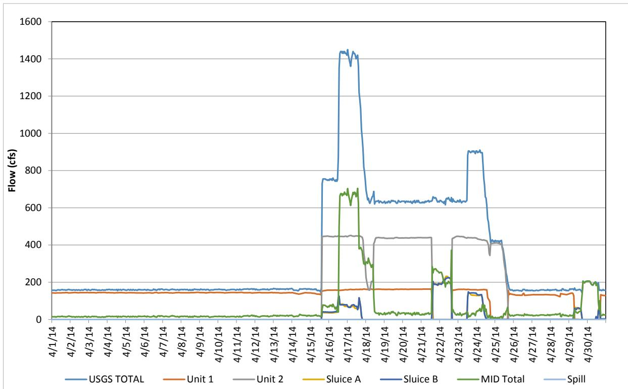
**Figure A-4.** Flow record in April 2014, based on hourly discharges.
