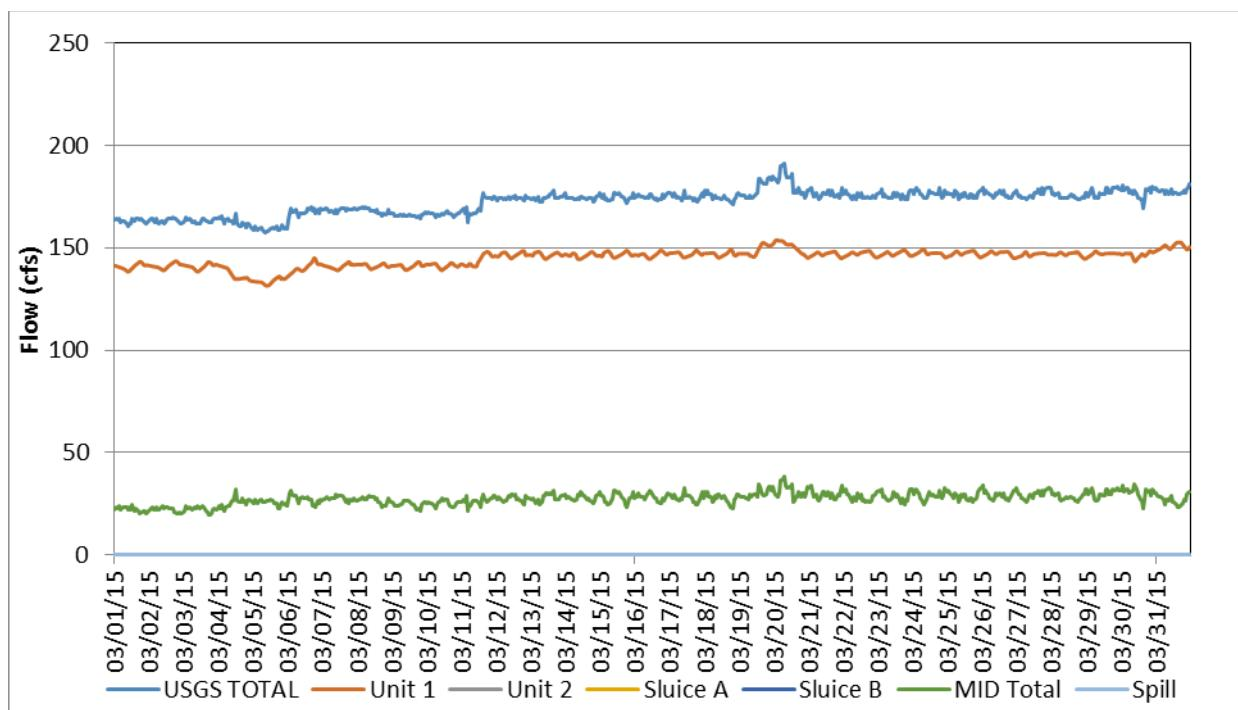
**Figure B-3.** Flow record in March 2015, based on hourly discharges.
